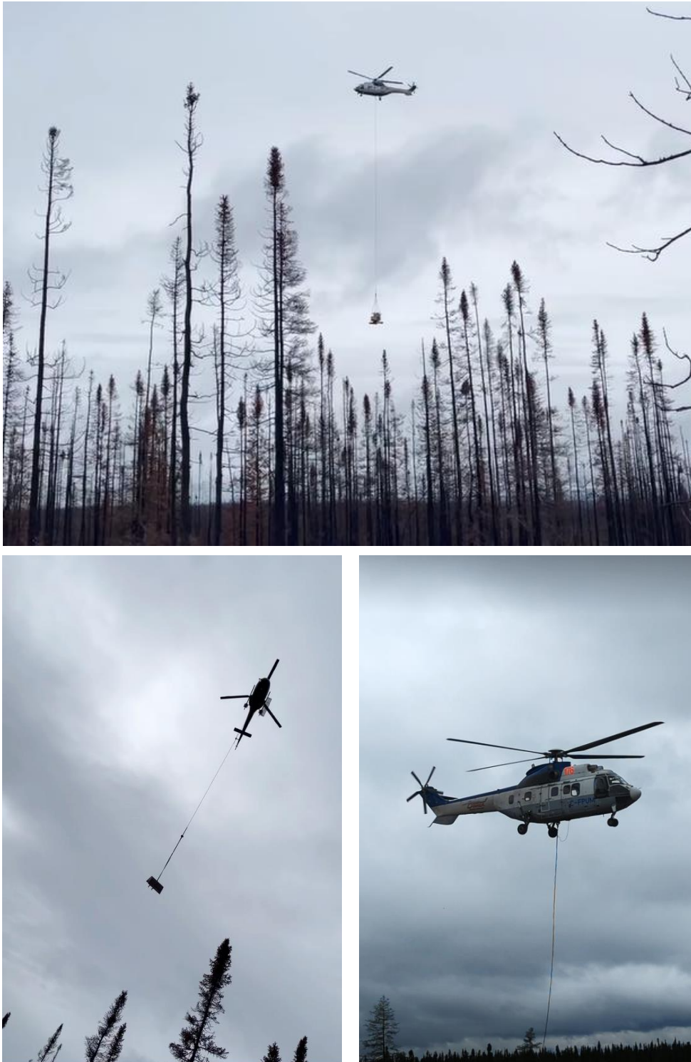
Figure 3: Super Puma helicopter active at Adina transporting drilling equipment and excavator.
