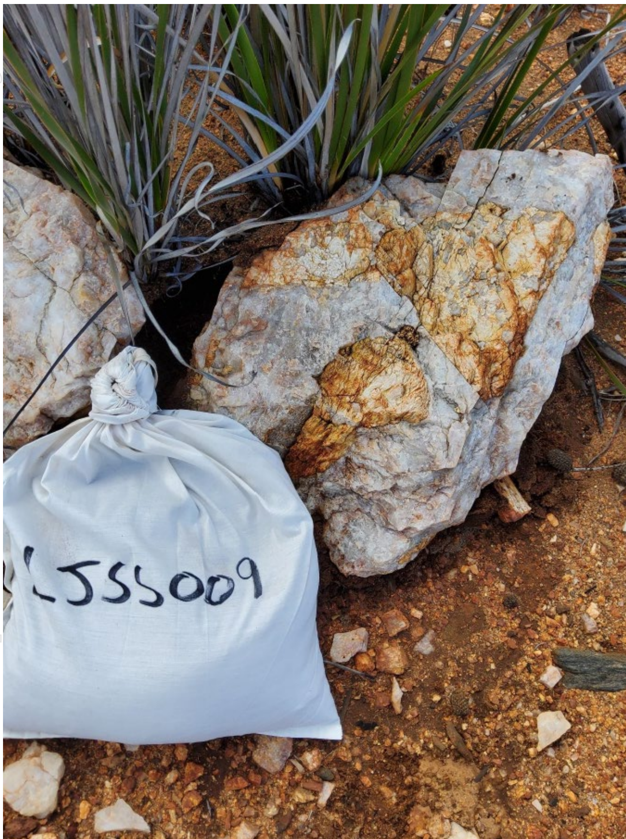
Figure 3 Outcropping very coarse pegmatite adjacent to soil sample LJSS009 with distinctive graphic quartz-feldspar texture.
