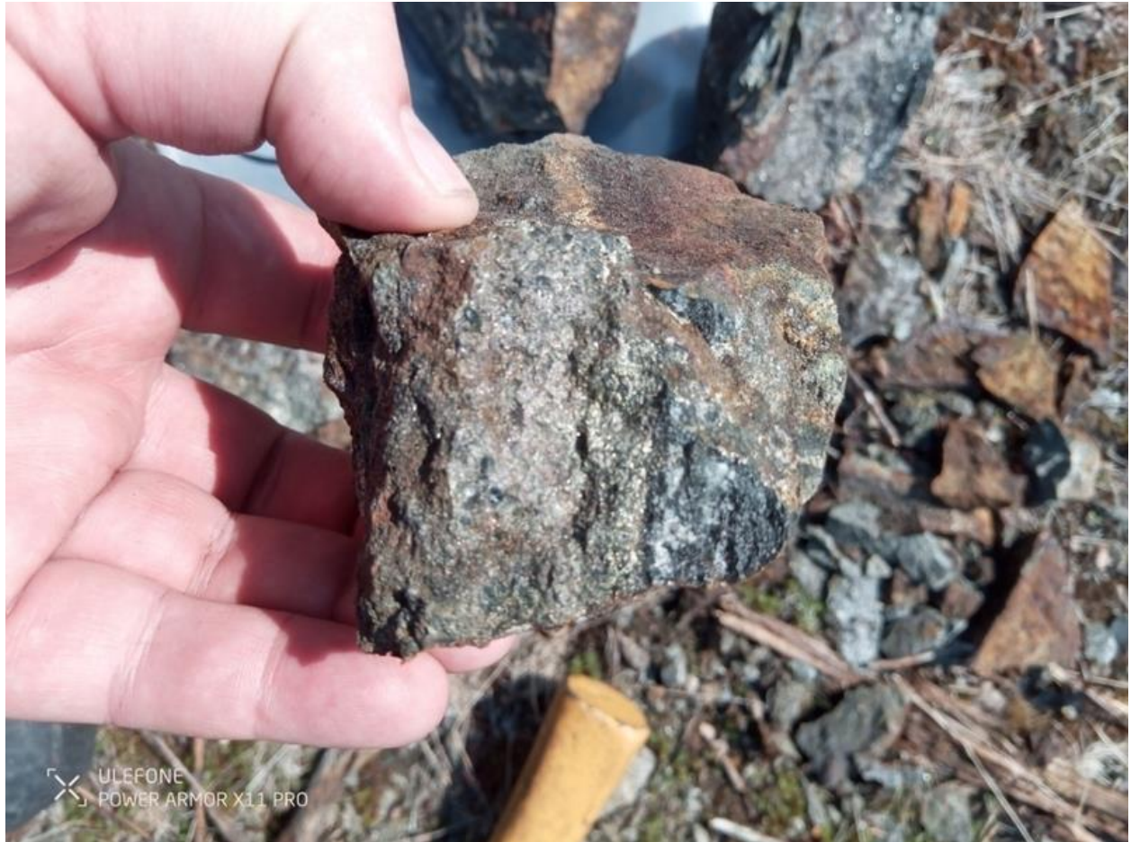
Figure 1 – Sample F0015010 – 3.48% Cu and >1% Ni – Semi-massive pyrite-pyrrhotite-pentlandite.
