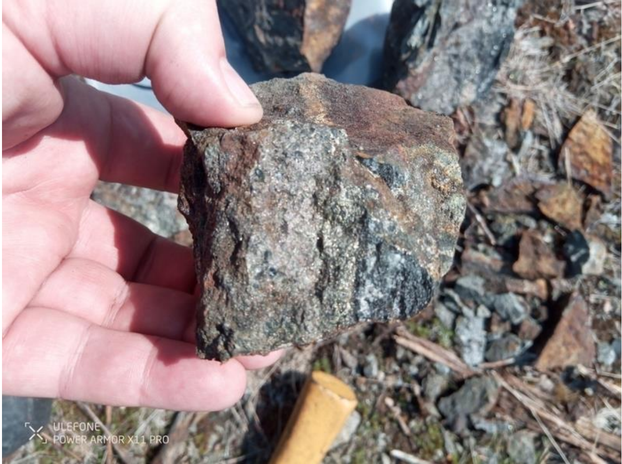
Figure 1 – Sample F0015010 – 3.48% Cu and >1% Ni – Semi-massive pyrite-pyrrhotite-pentlandite.
