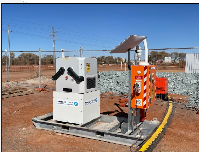
RocketDNA drone-in-a box installation on a client mine site in Western Australia
