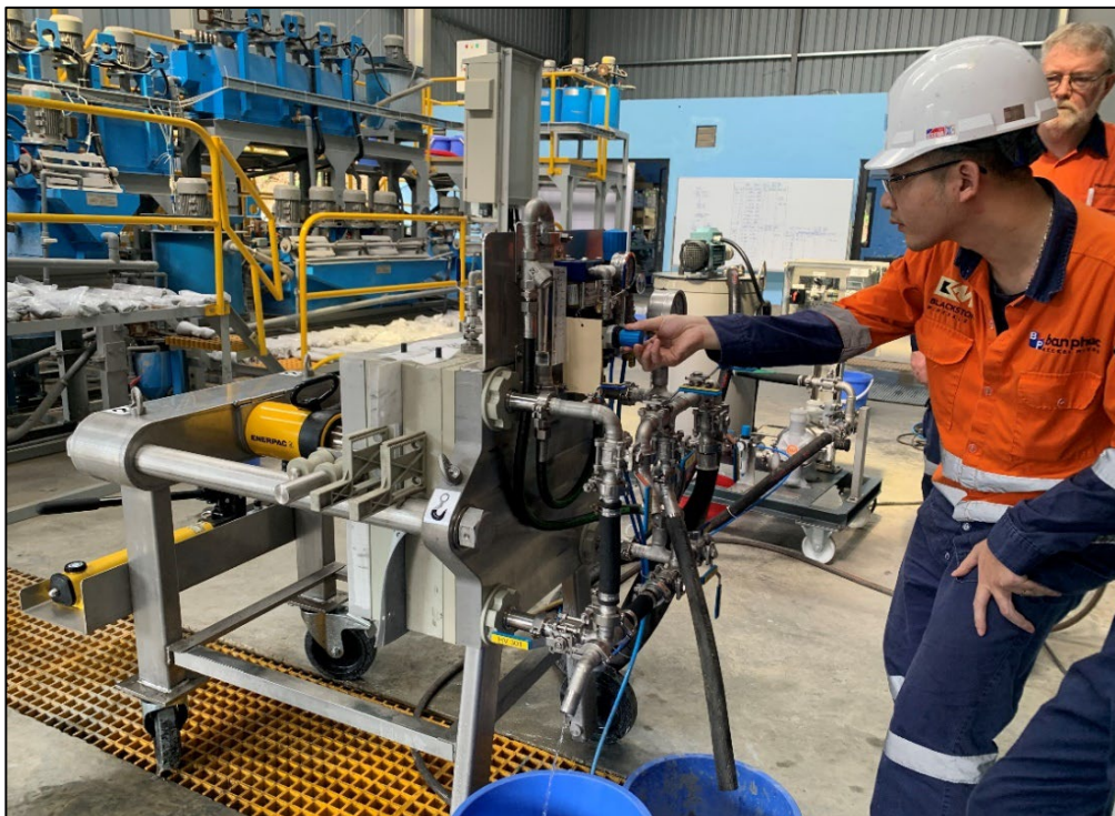
Figure 3 - Vendor piloting - Pressure filtration testwork trials
