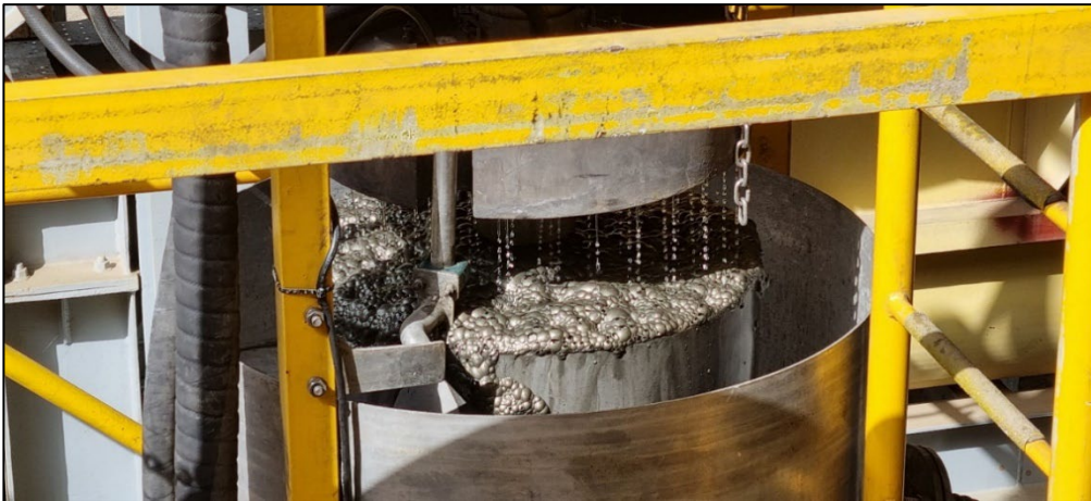
Figure 2: Vendor piloting - Jameson Cell trials producing improvements in Nickel and MgO concentrate grades
