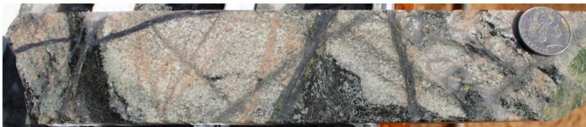
Figure 1: Porphyry-style alteration, veining and mineralisation in CPW0001DD at 594.66m. This section of HQ core is part of assayed interval 594.06 – 595.88 which returned 3936 ppm Cu and 745 ppm Mo for 0.92 % CuEq 1 .
