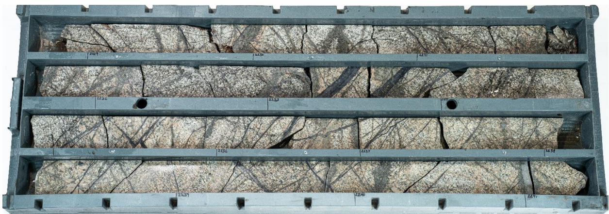
Figure 3: Drill core (HQ) from CPW0002DD showing similar style and intensity of stockwork quartz-sulphide veining as per CPW0001DD. The core in this photo is from 679.40 m – 683.06 m depth (2229' – 2241') part of logged interval 673.61 m – 694.03 m (2210' – 2277') which contains visually estimated 4% pyrite, 1% chalcopyrite and 0.4% molybdenite and 8 volume % quartz-sulphide veining.
