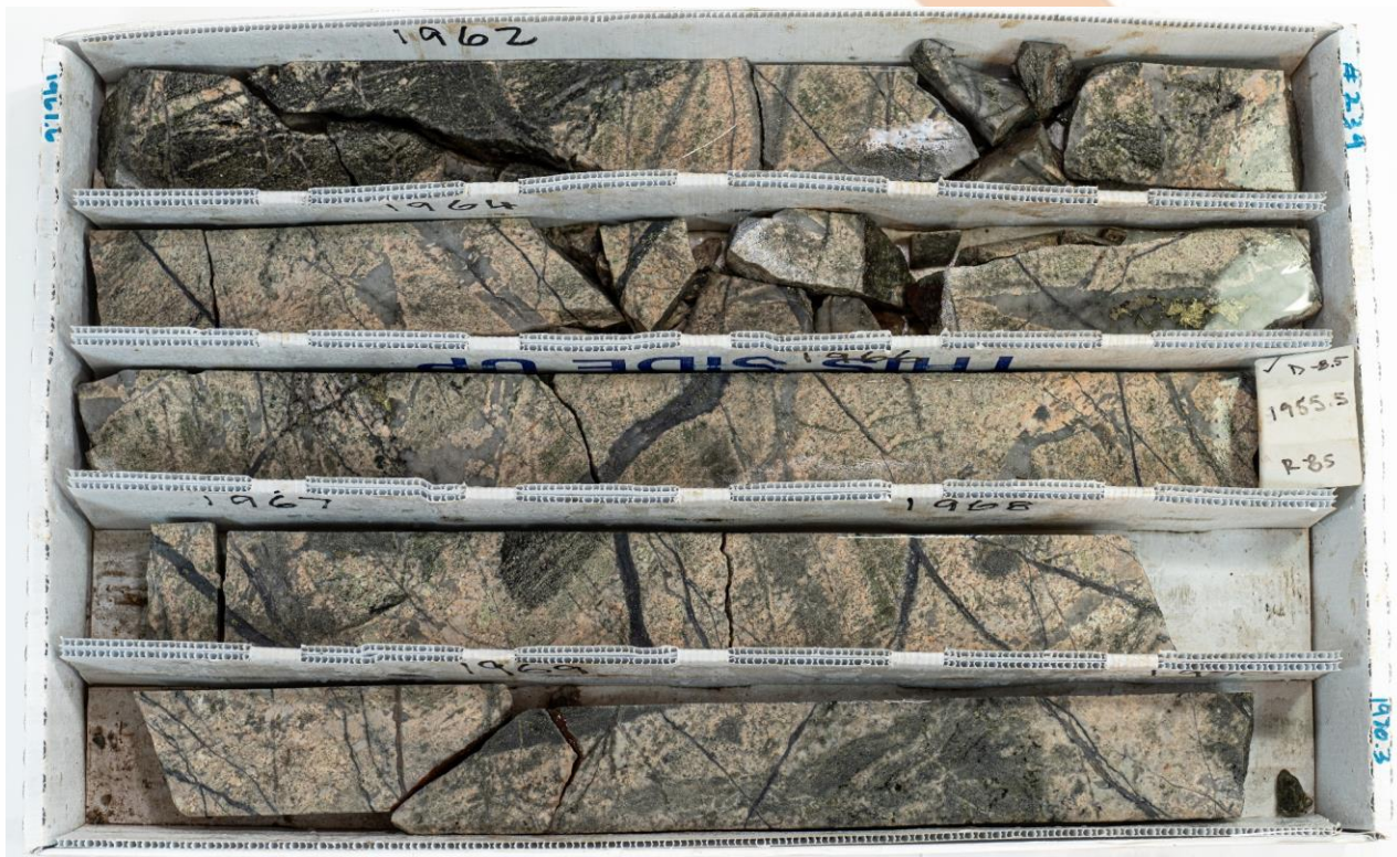
Figure 2: Drill core tray (HQ) from CPW0001DD showing high intensity of stockwork quartz-sulphide veining overprinting felsic gneiss and mafic schists. The upper section of HQ core in this photo is part of assayed interval 597.71 m – 599.54 m (1961' – 1967') which returned 7057 ppm Cu and 1295 ppm Mo for 1.62% CuEq 3 . The lower section of core is part of assayed interval 599.54 m – 601.37 m (1967' – 1973') which returned 2690 ppm Cu and 1509 ppm Mo for 1.33% CuEq 3 .
