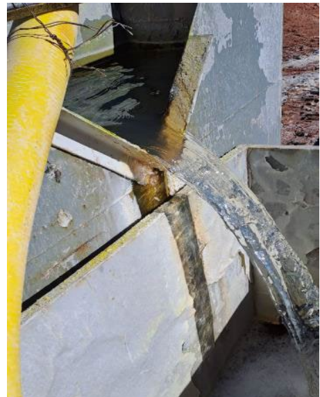
Figure 6: View of C-02-23 exploration well and ongoing airlift test.
