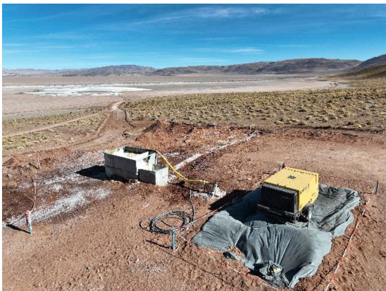
Figure 6: View of C-02-23 exploration well and ongoing airlift test.
