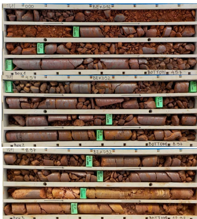
Figure 4 Drill core from drill hole BEKD092 High-grade DSO lump and fines iron ore product grading 66% Fe, from surface to 11.2 metres
