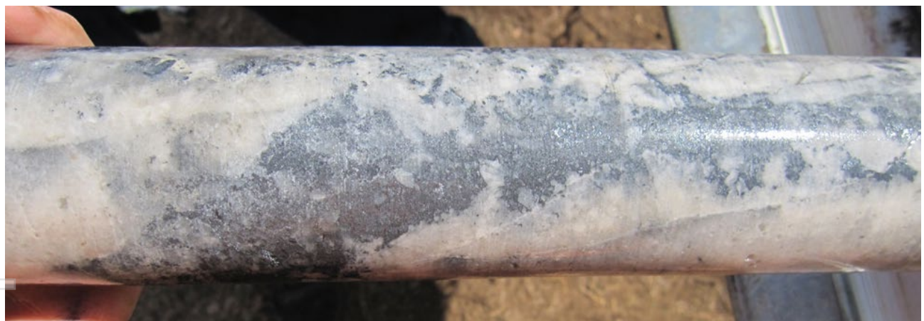
Figure 7-8. Banshee – drillhole CNDD01 illustrating antimony mineralisation in quartz.
