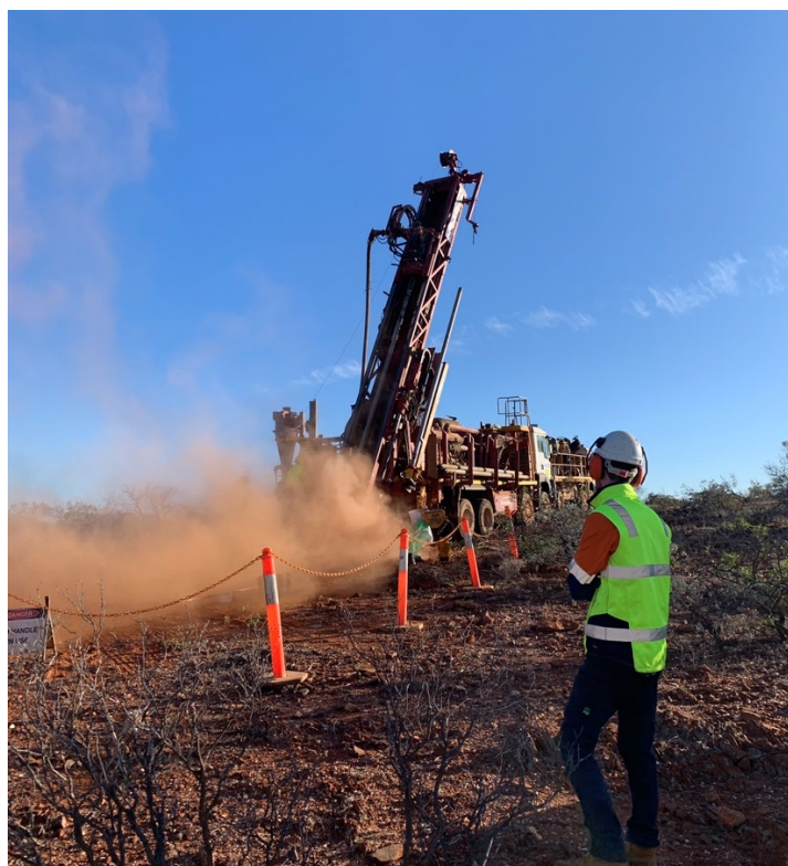
FIGURE 1: RC RIG DRILLING FIRST COLLAR AT JOHNSON'S WELL.
