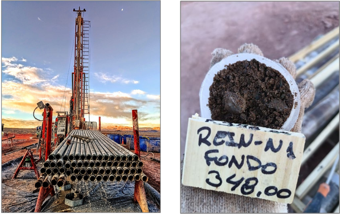
Figure 2. Diamond drilling rig at platform K23 and a representative gravelly sand from K23D40 at 348 m bgs
