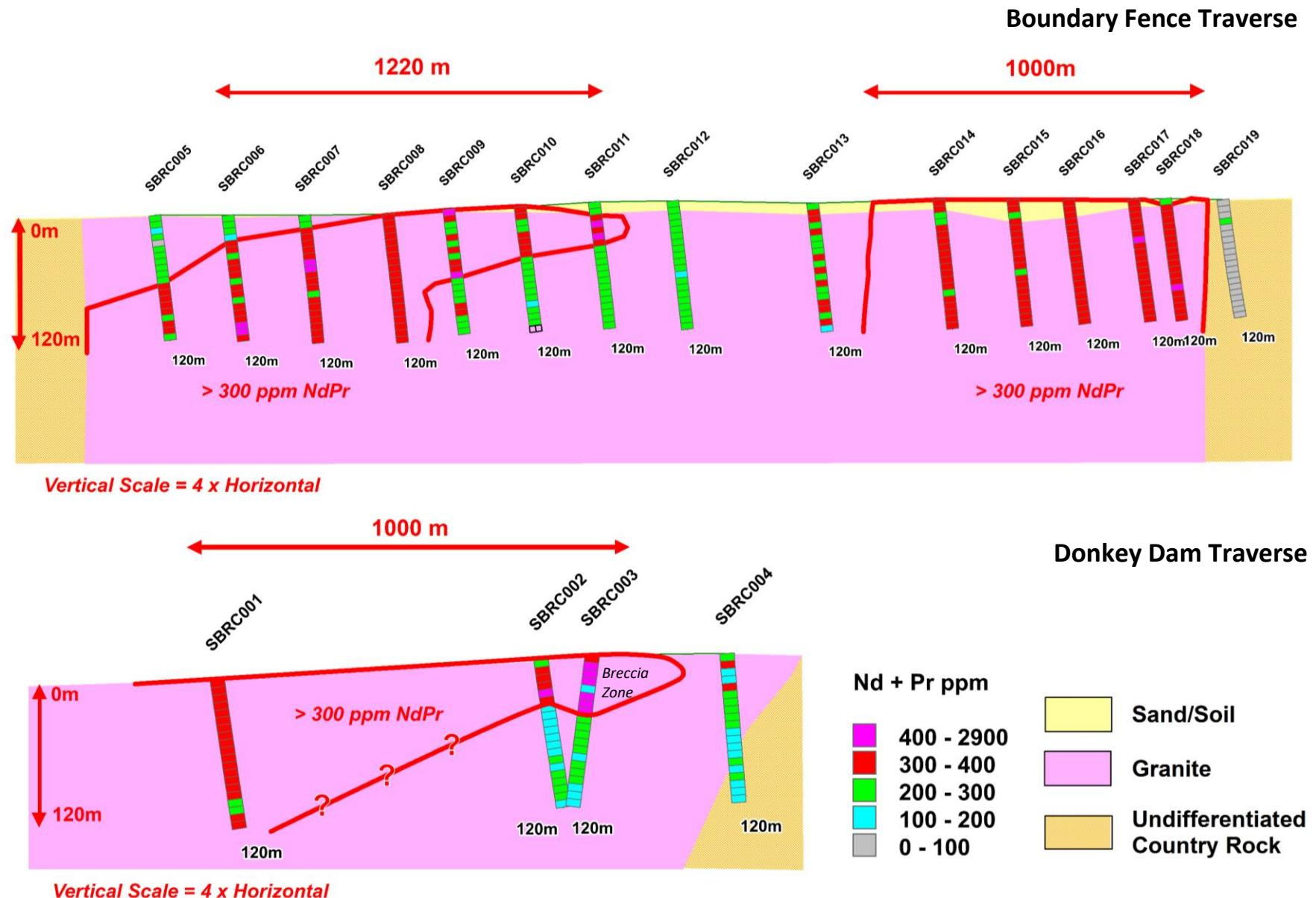
[Figure 2] Sybella Project: Drill sections showing variation in NdPr oxide values at depth and between holes for two traverses across the granite.
