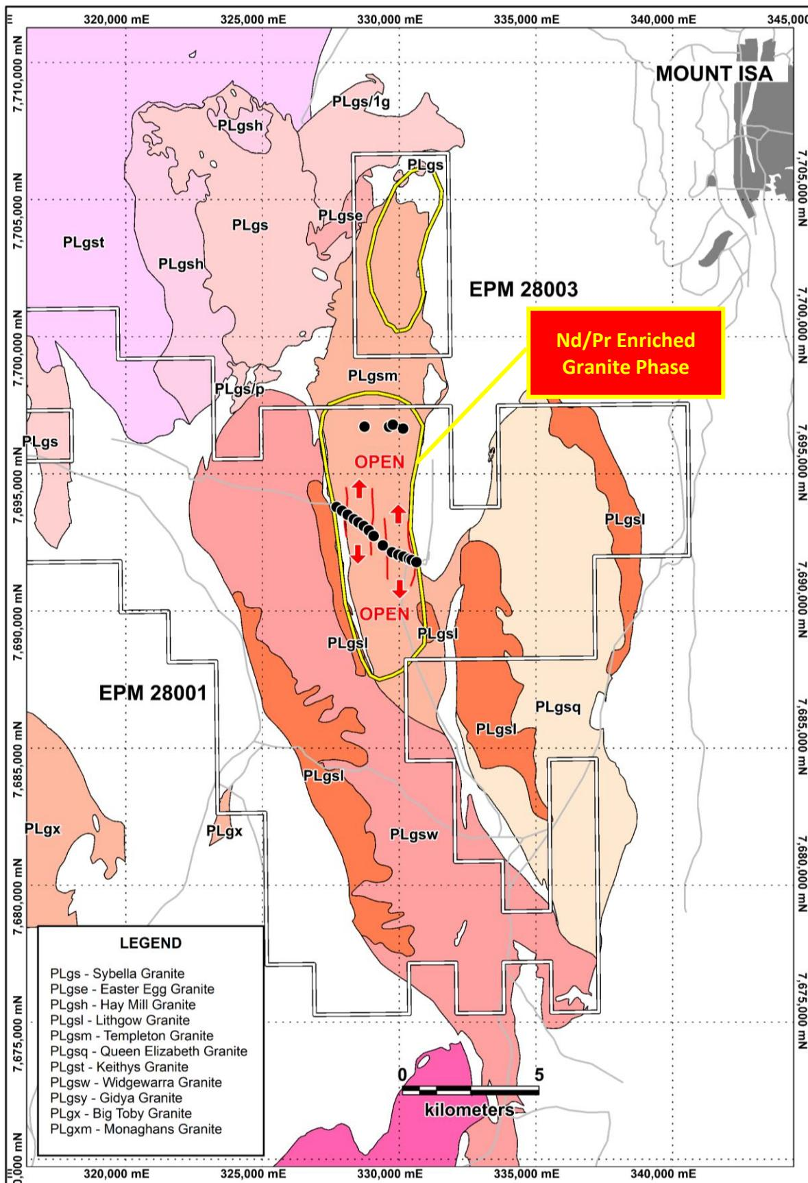
[Figure 3] Sybella Project: Red Metal 2023 percussion drill hole locations on a regional geological map highlighting multiple phases of granite intrusions. Note the interpreted extent of the REO enriched granite (yellow line) and wide zones of >300ppm NdPr (red).
