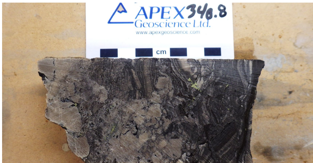
Figure 5: Blebby chalcopyrite (yellow brassy) and organic rich breccia in drill hole ST23-04 from approximately 340.8m downhole.
