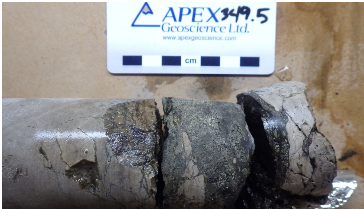
Figure 1: Breccia chalcocite (dark grey) and pyrite (yellow, brassy) in drill hole ST23-04 from approximately 349.5m downhole.
