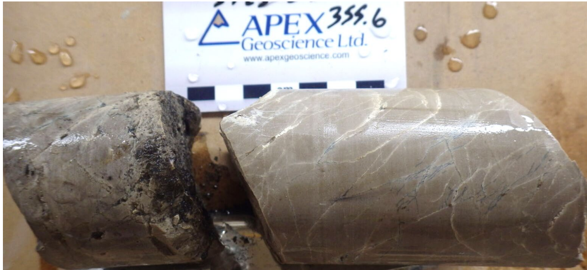
Figure 6: Breccia and veinlets of chalcocite (dark grey) in drill hole ST23-04 from approximately 355.6m downhole.
