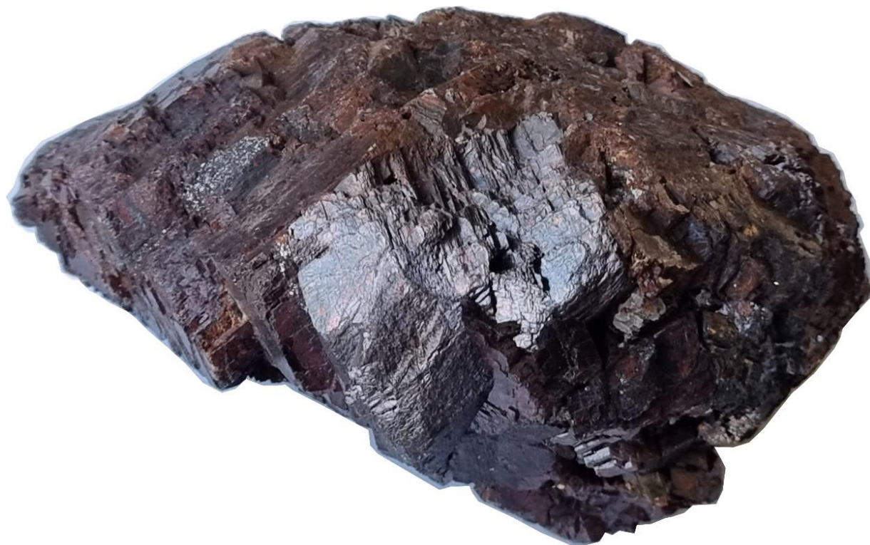
Figure 5. Mineralised waste dump specimen visually estimated to consist of 90% siderite and 10% cyrolite.
