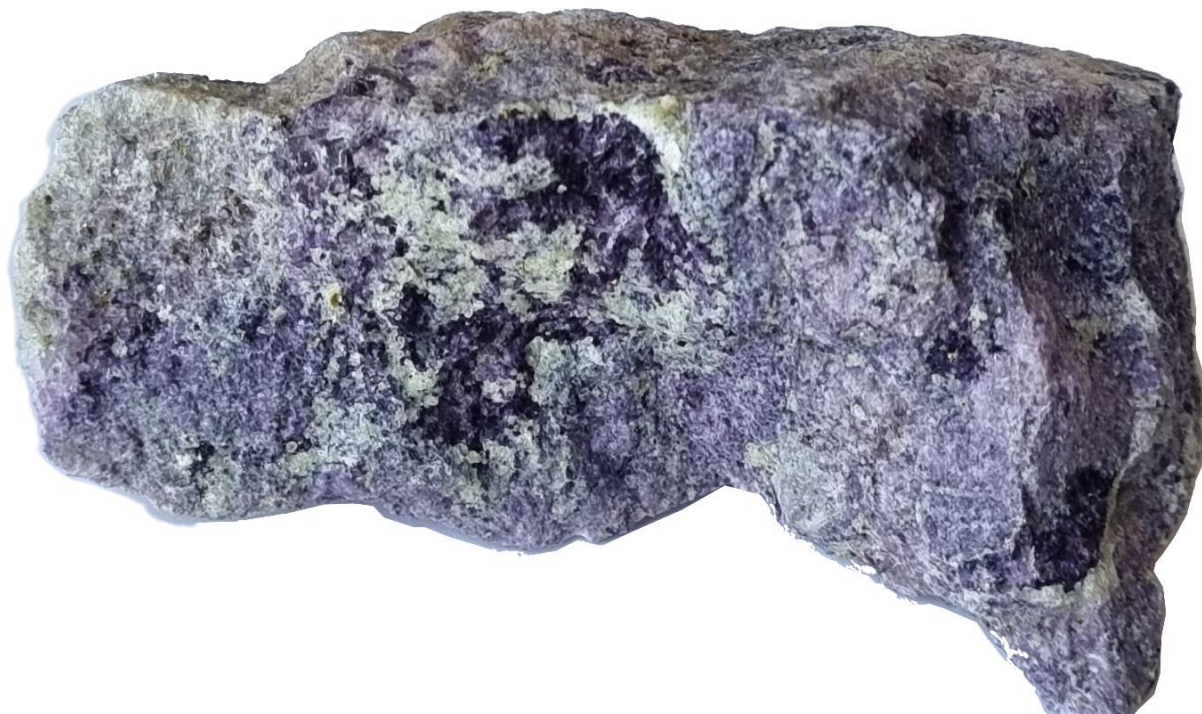
Figure 6: Mineralised waste dump specimen visually estimate to consist of 70% Purple Fluorite; 25% Green Fluorite; and 5% Cryolite.
