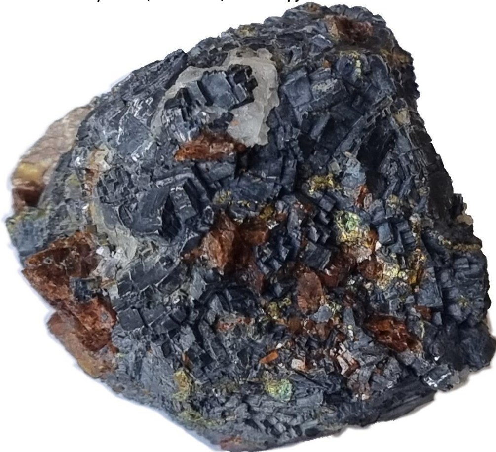
Figure 4. Mineralised waste dump specimen visually estimated to consist of 70% Galena; 10% Chalcocopyrite; 10% Sphalerite and 10% Quartz
