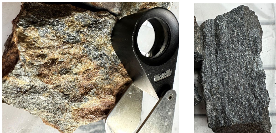
Figure 2: (left) photograph of pyrite (5%)-chalcopyrite (2%)-altered rock from Morkens Prospect that returned 19.7% TREO and 169 g/t Ga in sample 23GRUGS013; & (right) magnetite-rich rock that assayed 32% Fe 2 O 3 , 1433 ppm TREO and 10 g/t Ga in sample 23GRUGS008.
