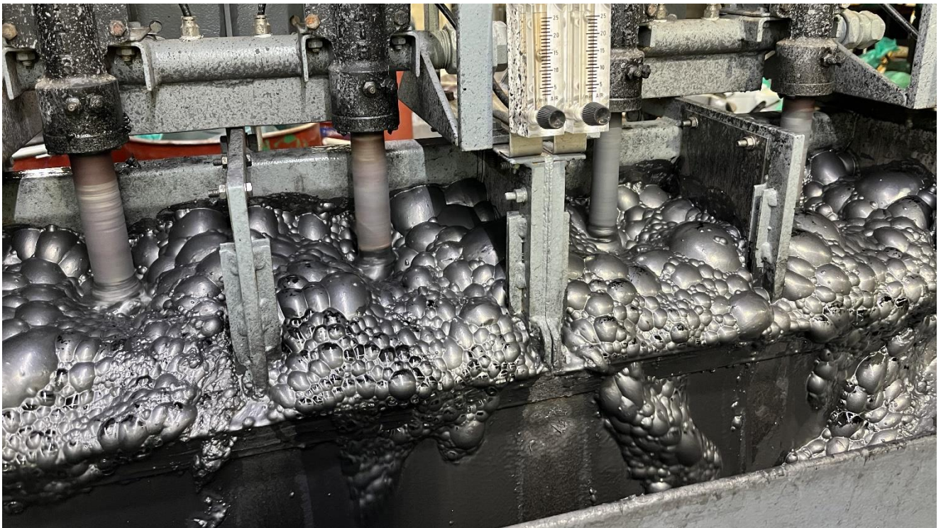
Figure 1 – Rougher stage of bulk flotation test on Sarytogan Graphite underway at IMO in Perth, Australia, August 2023.
