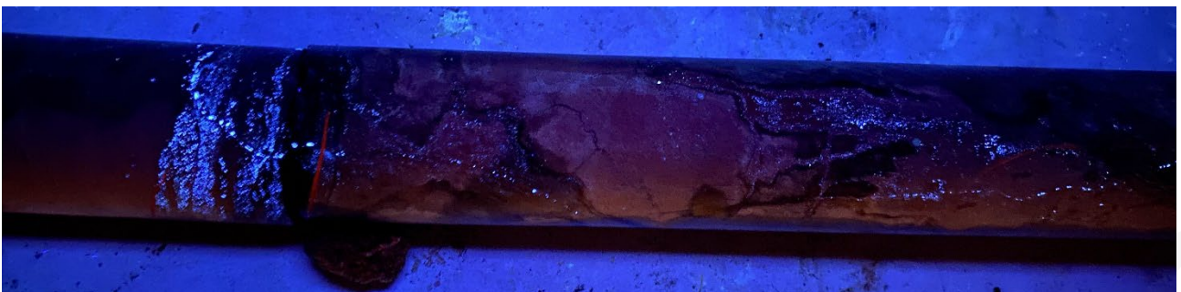
Figure 7. KI 112, 334.2m garnet-pyroxene skarn and scheelite ultraviolet light.
