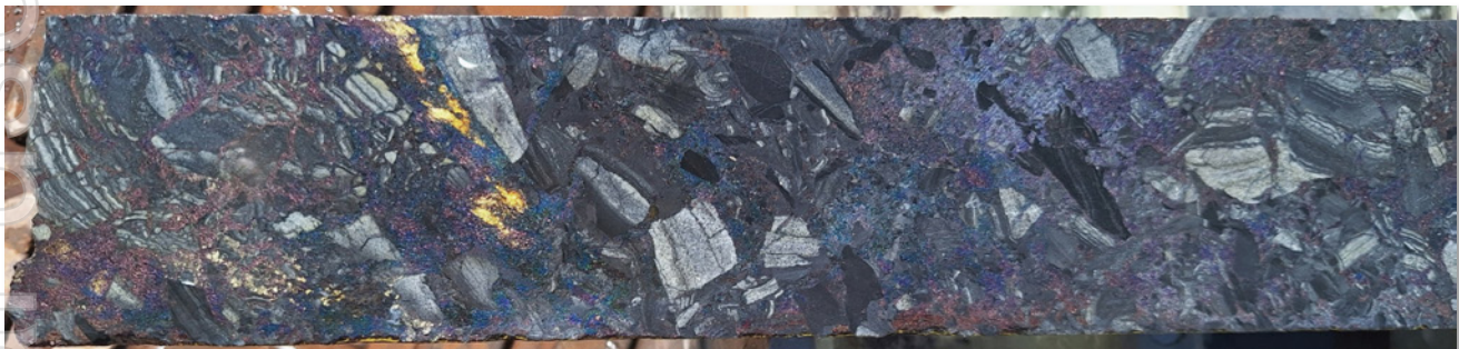
Figure 1: High-grade chalcocite, covellite, bornite & chalcopyrite sulphide matrix breccia. 1.10m @ 24.8% Cu, 93.2 g/t Ag and 1,125 ppm Co from within the 66.50m (48.00m*) @ 4.95 % Cu, 32.7 g/t Ag and 686ppm Co from 234.00m^
