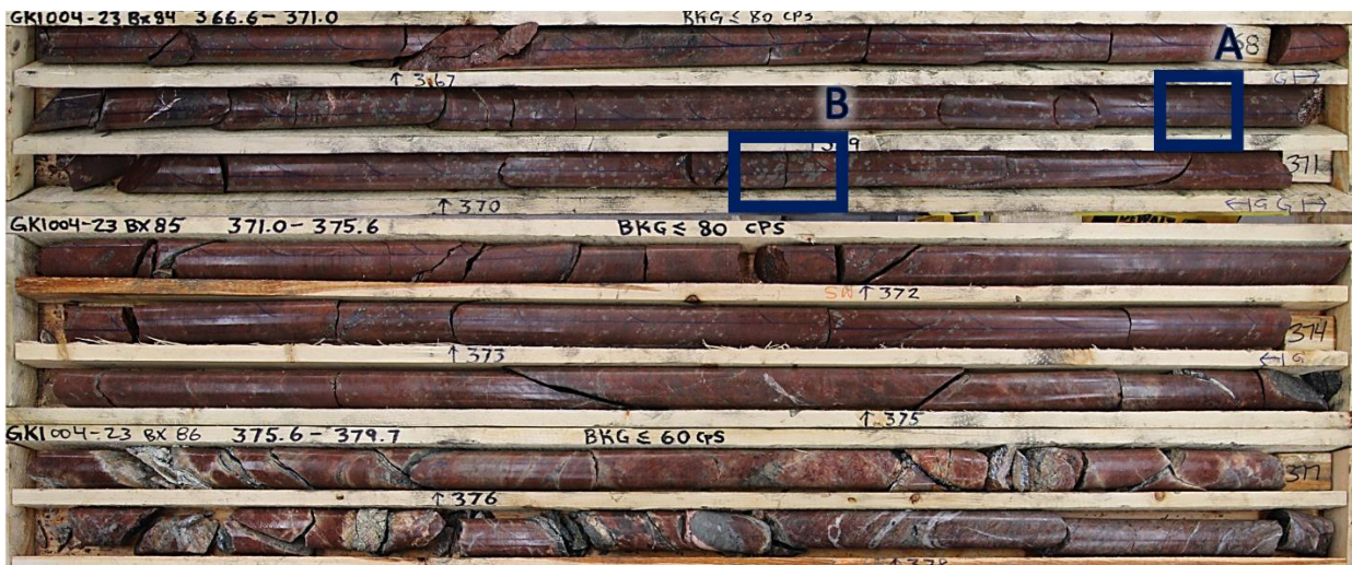
Figure 4: Close-up of strongly fractured hematized interval intersected in drillhole GKI-004. Deformation is characterized by an extensive network of microfractures, open fractures, quartz veins, cohesive dark green cataclastic bands and incohesive centimetre scale breccias and gouges. A bleaching halo is commonly observed peripheral to the fractures and microfractures planes and gritty white fine grained clay matrix is noted in the incohesive breccia and gouges.
