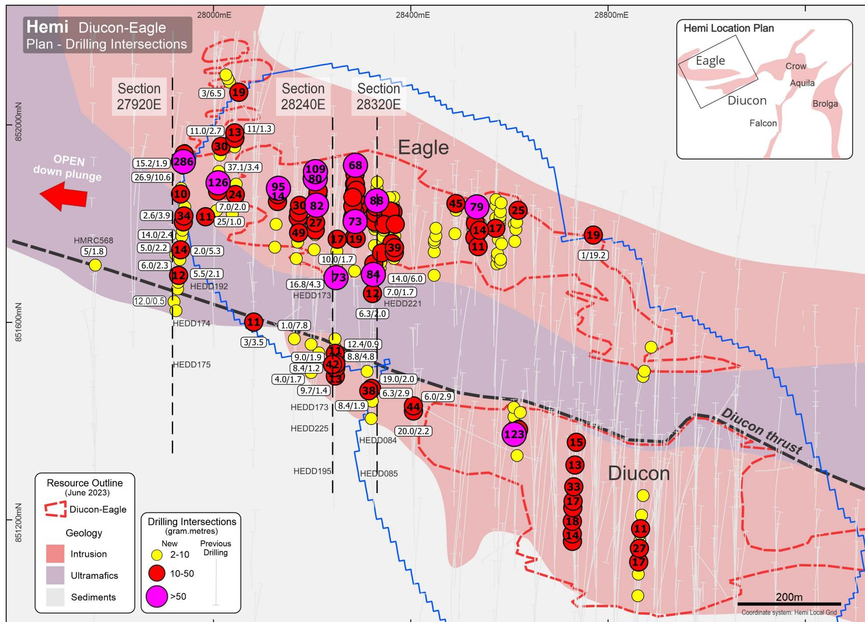
**Figure 3 Eagle Long Projection showing new drill results outside preliminary open pits**
