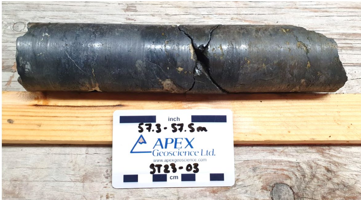
Figure 4: Massive chalcocite (dark grey) in drill hole ST23-03 from approximately 57.4m downhole.
