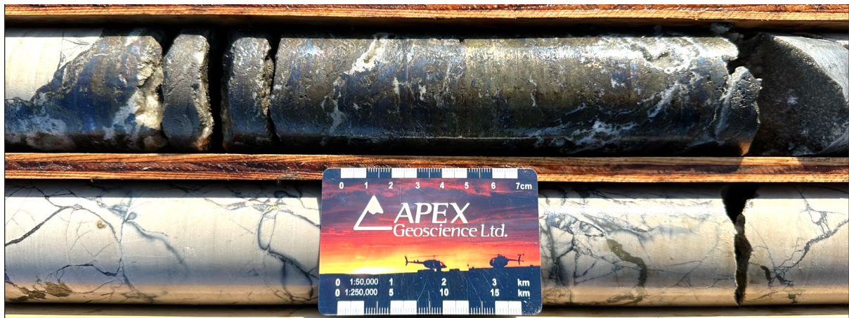
Figure 1: Massive chalcocite (dark grey) and chalcopyrite (brassy) in drill hole ST23-03 from approximately 58m downhole.
