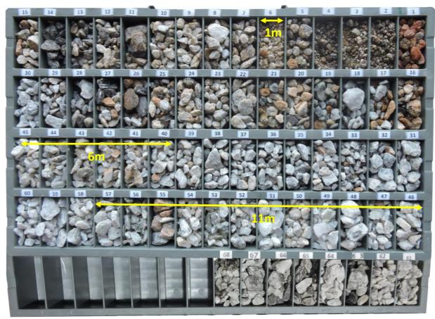
**Photo 3** – Example of chip tray from SOL-RC-08 (Zilcar II). Yellow arrows = pegmatite intercepts
