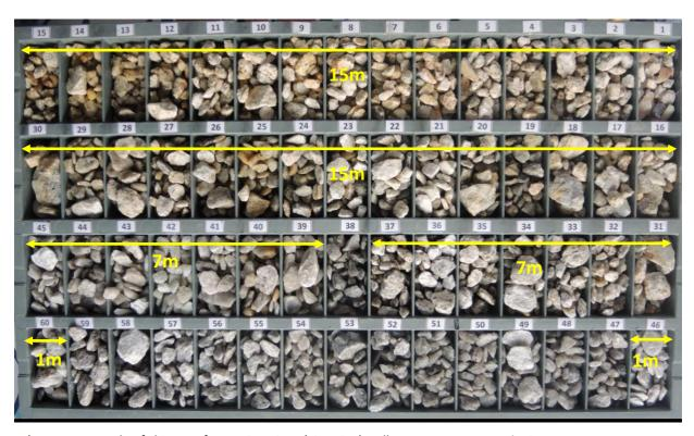
**Photo 1** – Example of chip tray from NGR-RC-15 (Tin Mine). Yellow arrows = pegmatite intercepts
