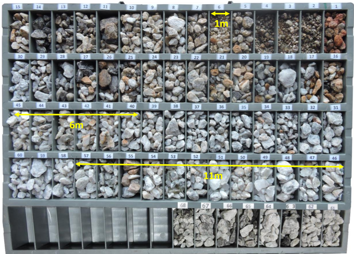
Photo 3 – Example of chip tray from SOL-RC-08 (Zilcar II). Yellow arrows = pegmatite intercepts
