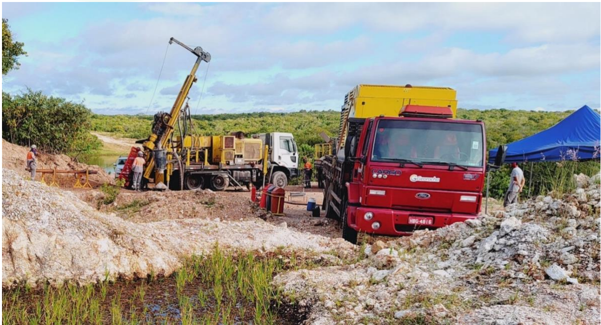
Photo 6 – NGR RC 007 – drilling RC Inclined Hole
