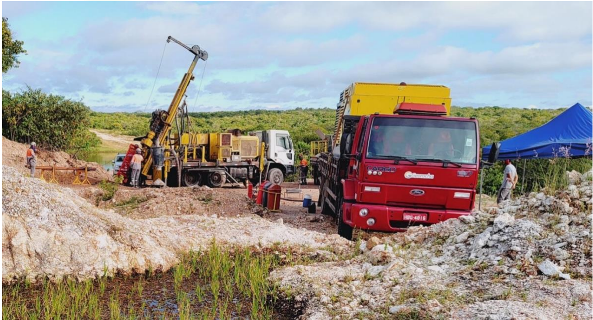
Photo 6 – NGR RC 007 – drilling RC Inclined Hole
