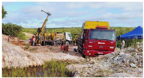
**Photo 6** – NGR RC 007 – drilling RC Inclined Hole
