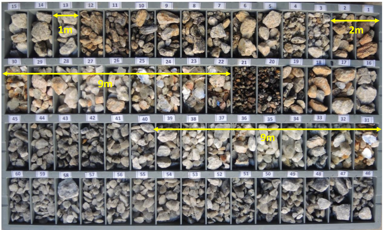
Photo 2 – Example of chip tray from SOL-RC-06 (Zilcar II). Yellow arrows = pegmatite intercepts
