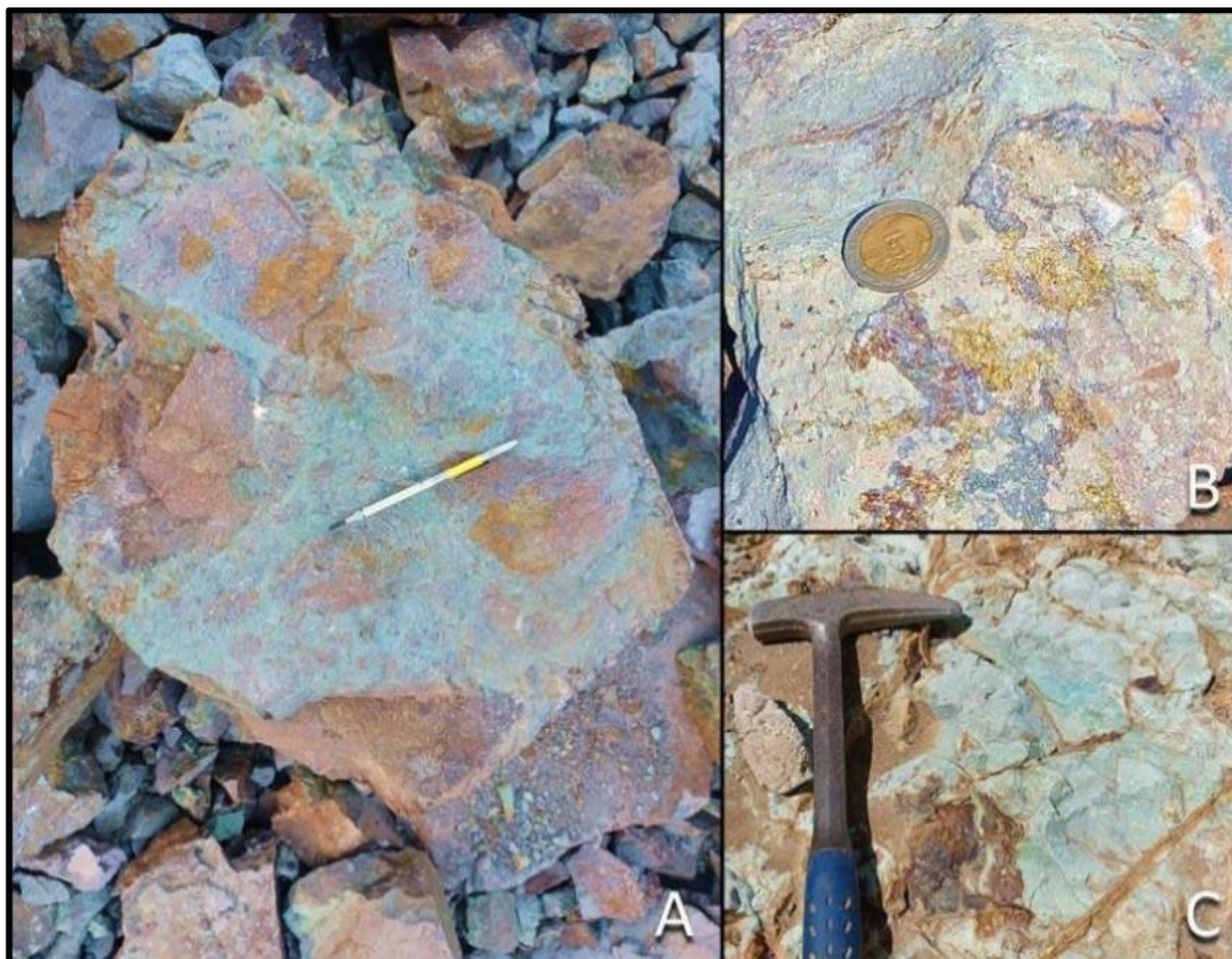
Figure 3: (A) Outcropping breccia hosted copper mineralisation at Vaca Muerta, (B) Bornite and chalcopyrite mineralisation present in stockpiles at El Quillay (C) Outcropping copper oxide mineralisation associated with an extensive stockwork and alteration zone (1300m x 400m) at La Florida.
