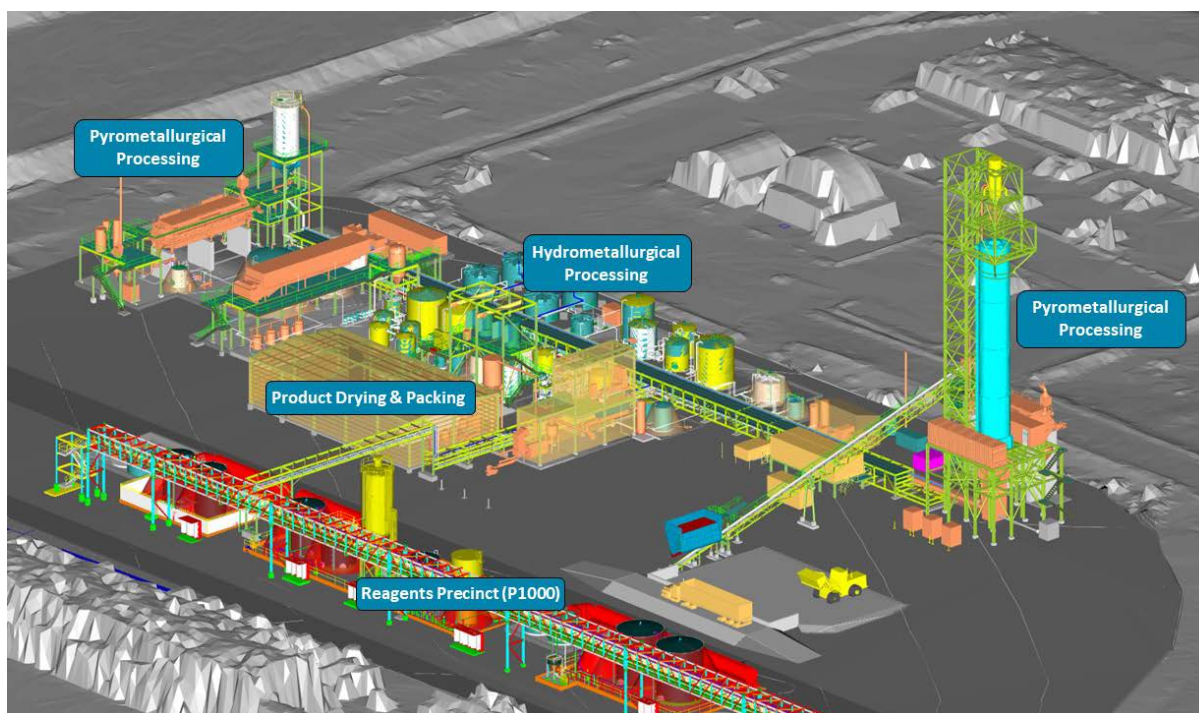
Figure 2 – Mid-Stream Demonstration Plant location and layout
