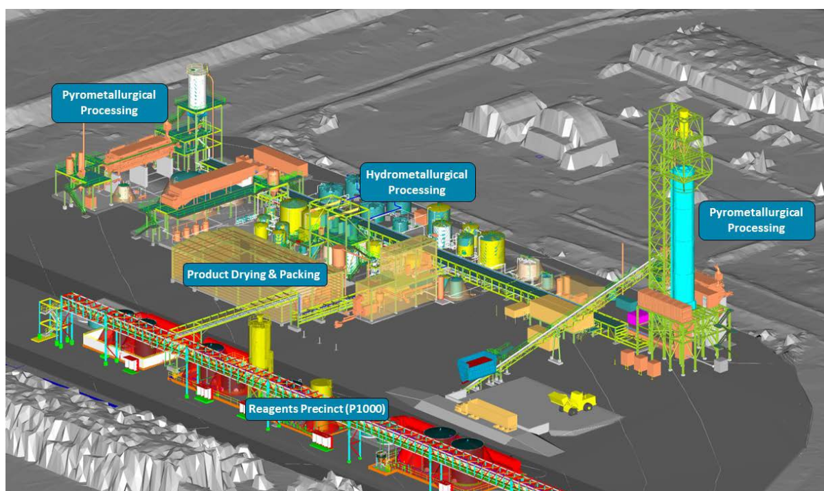
Figure 2 – Mid-Stream Demonstration Plant location and layout
