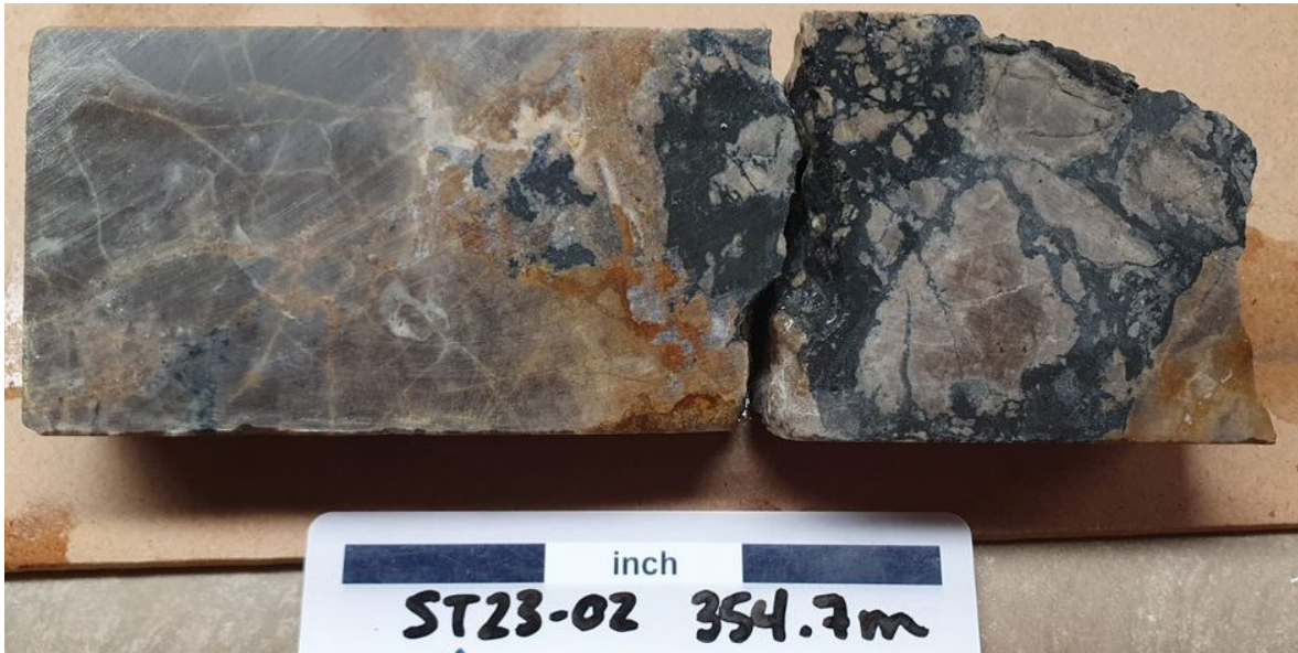
Figure 5: Chalcocite (dark grey) breccia fill in drill hole ST23-02 from approximately 354.7m downhole.
