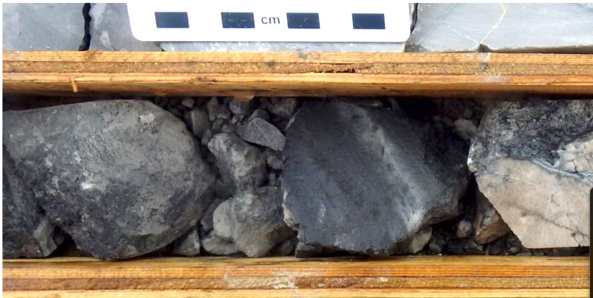
Figure 10: Dense veins of chalcocite (dark grey) in drill hole ST23-01 from the 4100N Zone. The drill core shown is from approximately 76m downhole.
