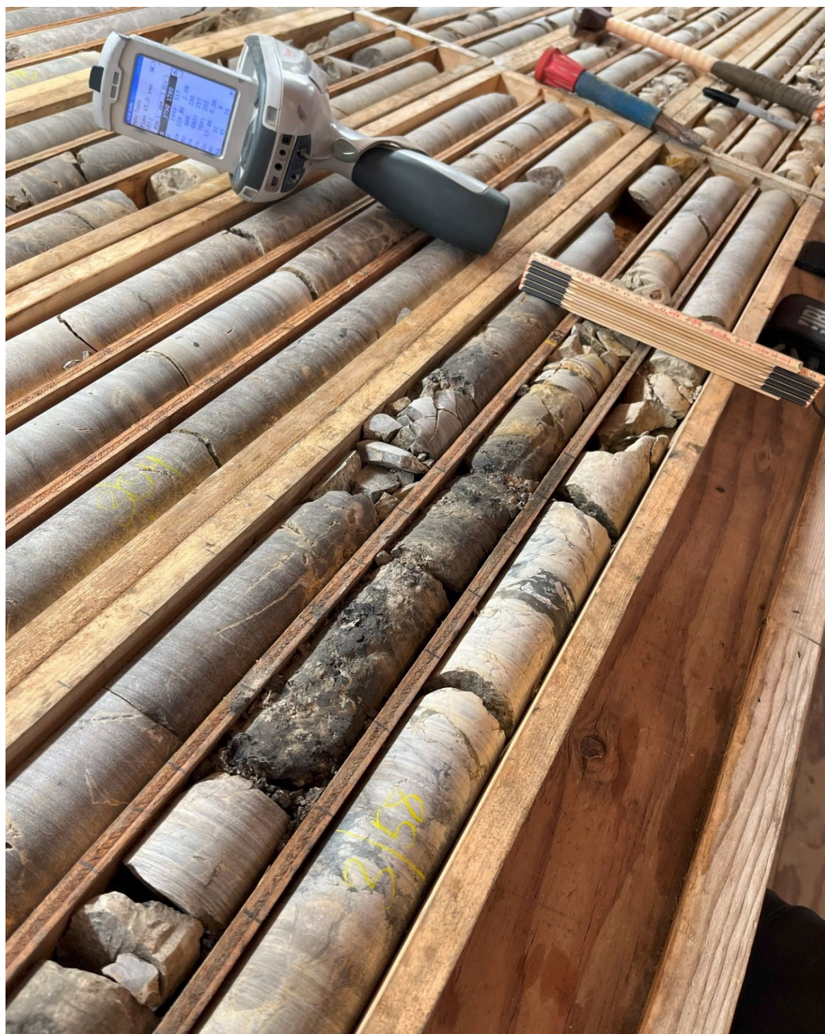
Figure 6: Chalcocite (dark grey) breccia fill in drill hole ST23-02. The interval shown is approximately 352-359m downhole.
