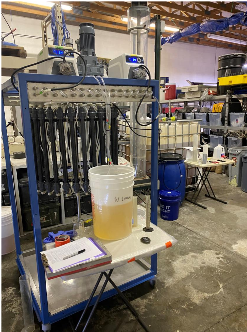
Figure 2: The benchtop Direct Lithium Extraction (DLE) setup in the independent laboratory in Salt Lake City.
