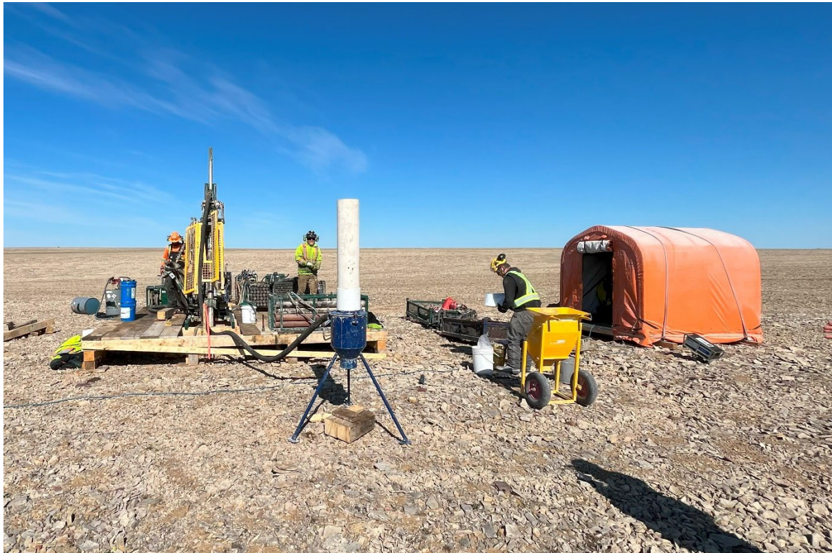
Figure 1: Reverse Circulation (RC) ‘Hornet’ drilling rig set-up at the 4100N Zone, Storm Project.
