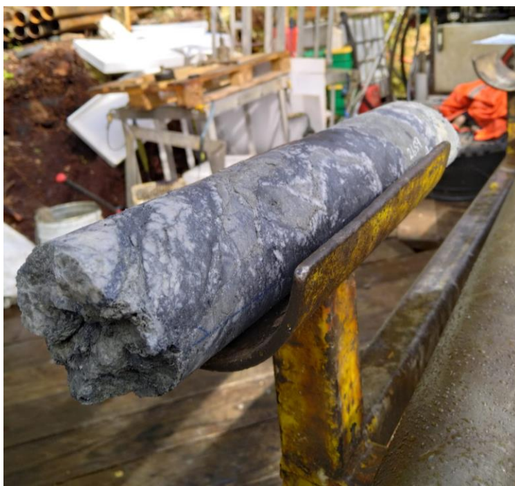
Figure 7. Stibnite (black) cemented host rock breccia from ACDDH004 at 131.4 to 131.8m that assayed 6.7/t Au, 20.9% Sb for 56.0g/t AuEq.
