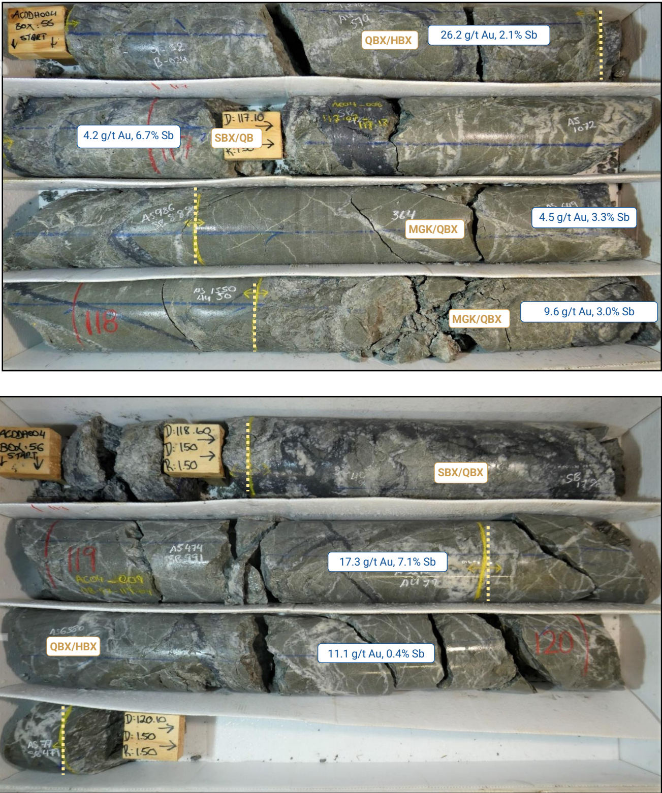
Figure 8. Fraternal Shoot intersected in AXDDH004 from 116.2m – 120.1m (SBX - stibnite cemented breccia, QBX – quartz breccia, HBX – host rock breccia, MGK – silicified disseminated arsenopyrite mineralised greywacke, MAR - silicified disseminated arsenopyrite mineralised argillite).
