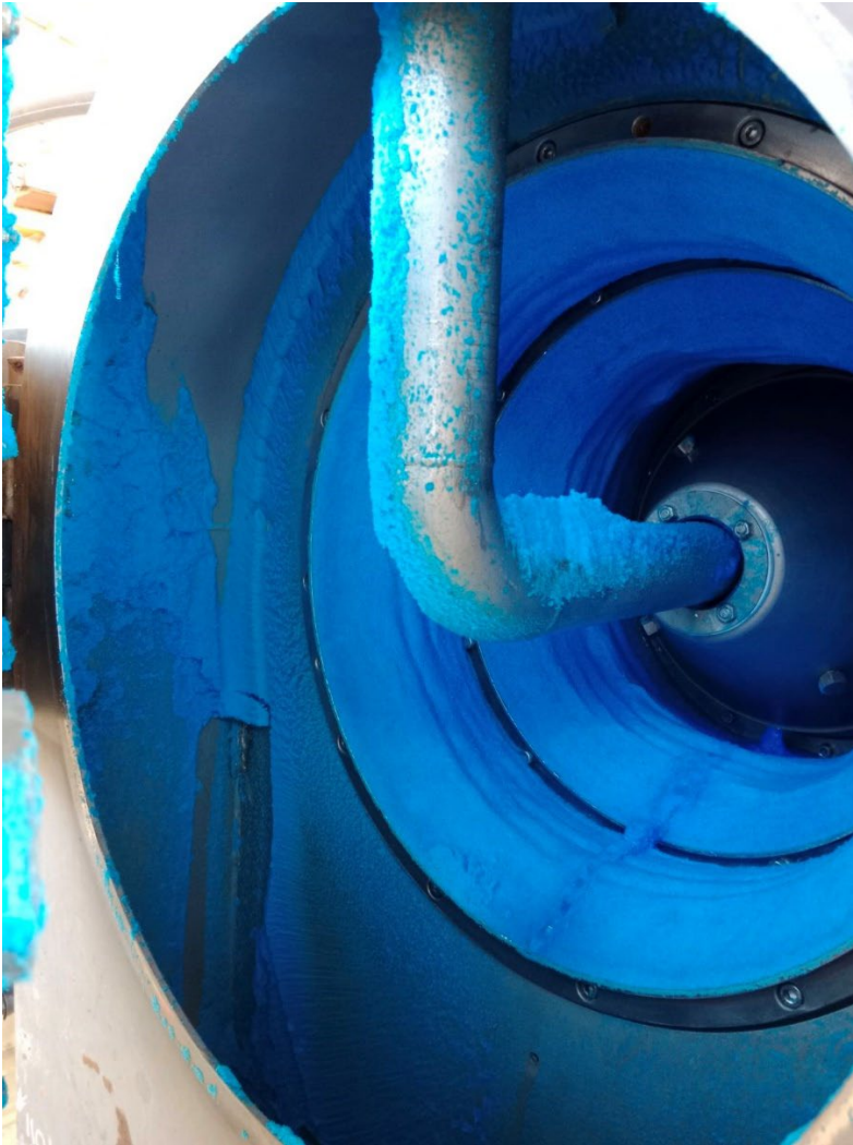
Figure 2: Picture of the centrifuge loaded with copper sulphate crystal produced at the Cloncurry Project Copper Sulphate Plant
