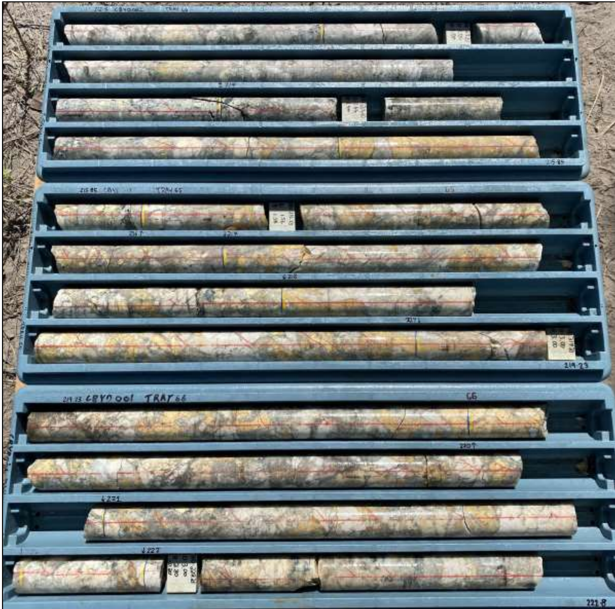
Photograph 1. Drill core from hole CBYD001 from 212.5m – 222.8m showing pegmatite with visually estimated spodumene content between 3% and 12%. 9
