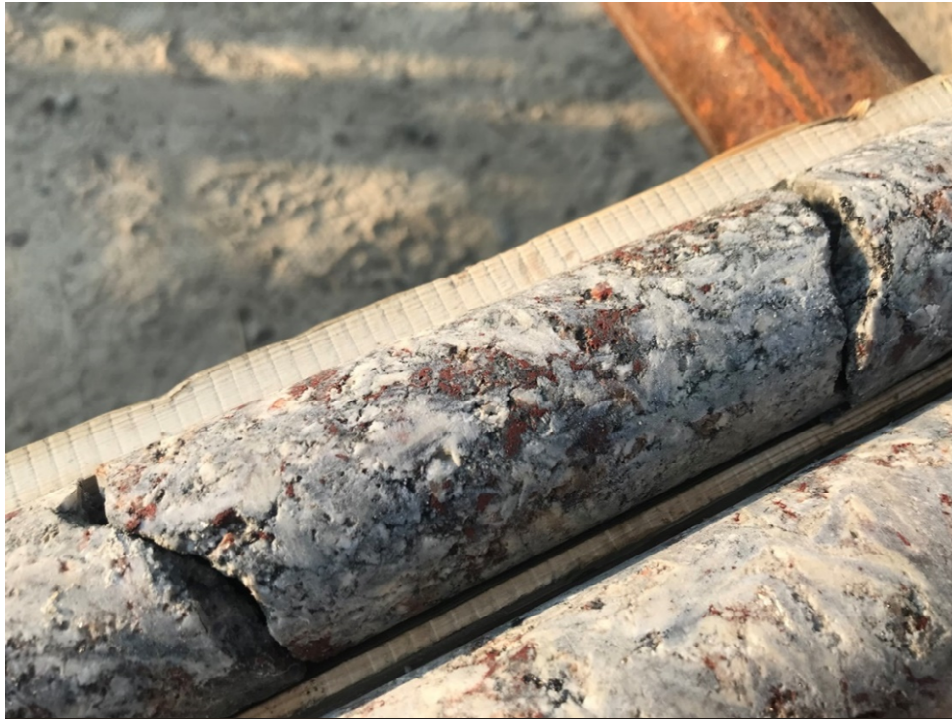
Figure 8: Diamond drill core (NQ, approximately 4.8 cm diameter) containing REE mineralisation (red coloured disseminations) within ferrocarnatite host rock. Hole POM-23-01, Box 104, 475.6 – 479.9 metres downhole depth.
