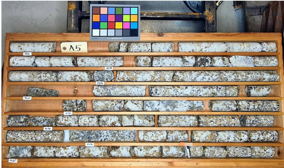
Figure 5. Diamond drill core from Hole A, upper zinc zone (approximately 26.8 to 35.2m down hole), showing siderite and sphalerite mineralisation in a quartz host with black marmatite, an iron-rich variety of sphalerite.
