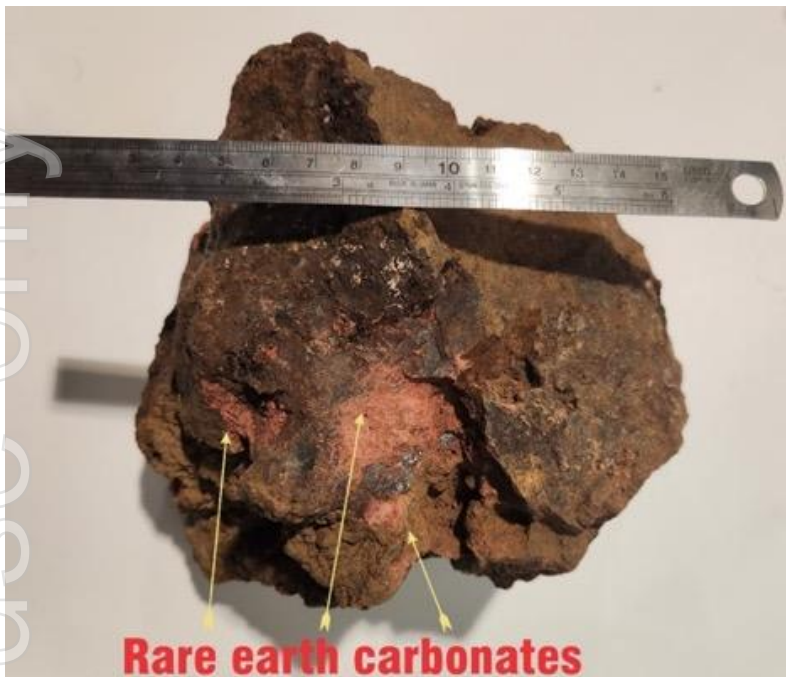
Figure 7: Grønnedal surface sample shows pink/orange REE mineral. Visually estimated to comprise of ~25% pink-orange material and 75% iron oxides and oxidised carbonatite.
