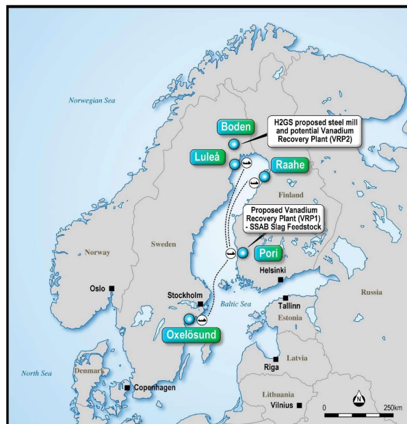
Figure 9: Map showing potential Vanadium Recovery Plants (Pori (SSAB Feed) and Bodén (H2GS Feed)) and SSAB Slag stockpiles
