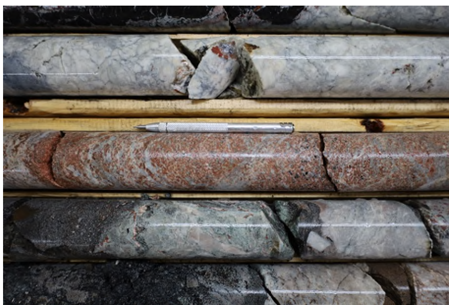
Figure 4: Diamond drill core (NQ, approximately 4.8 cm diameter) containing strong REE mineralisation (red coloured disseminations to semi-massive) within ferrocyanatite/calcioyanatite host rock. Hole POM-23-03, 173 metres downhole depth.
