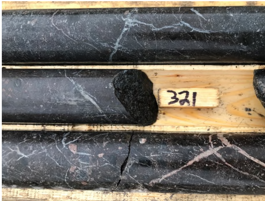
Figure 3: Diamond drill core (NQ, approximately 4.8 cm diameter) containing REE mineralisation (reddish-brown coloured blebs and within veins) within magnetic silicocarbonatite host rock. Hole POM-23-02, 321 metres downhole depth.
