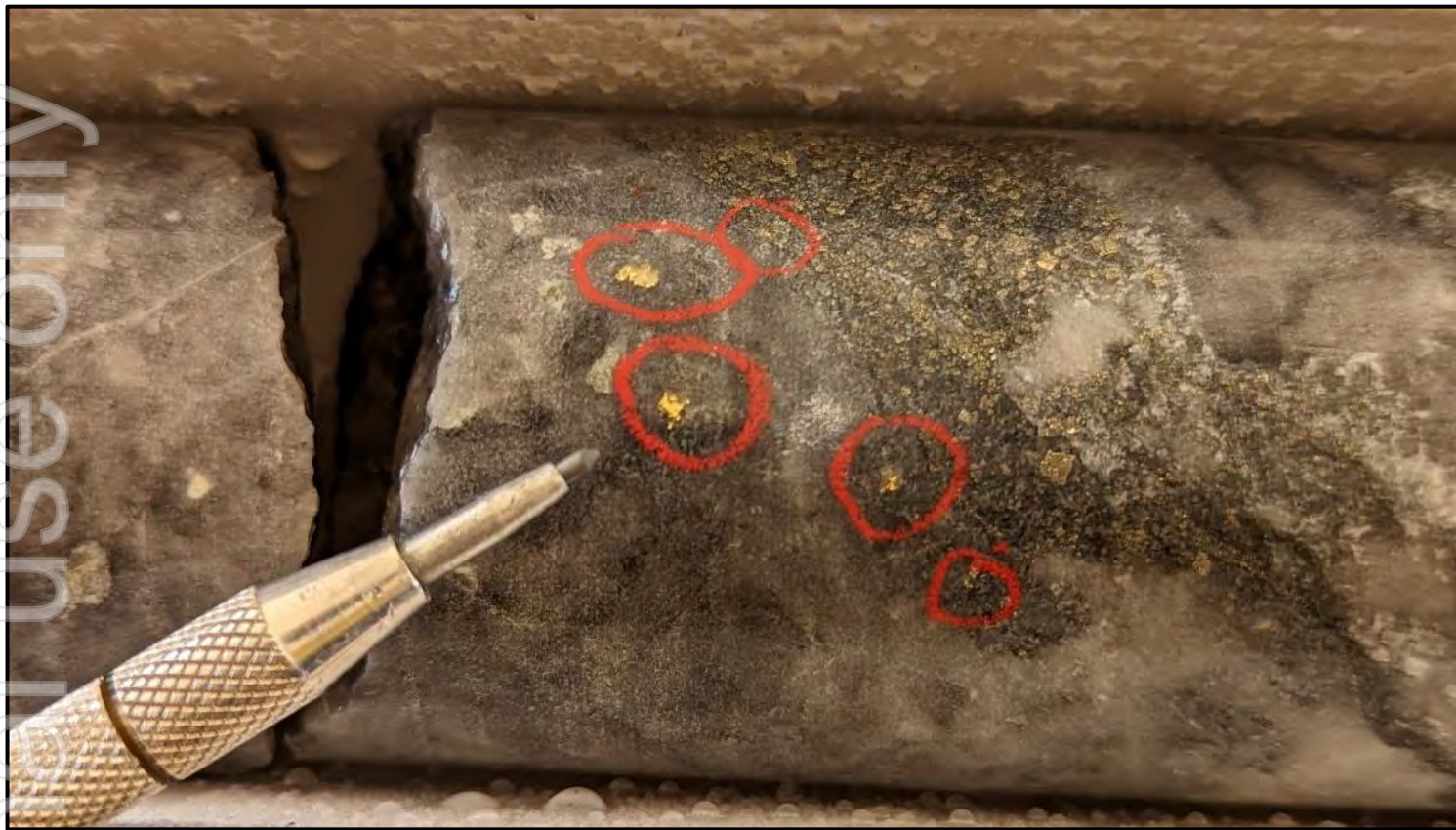
Below Diucon pit shell – visible gold in smokey quartz vein at 741m in HEDD136
