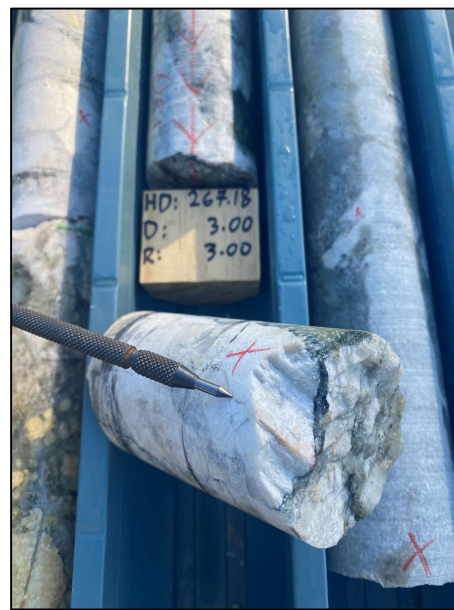
Photograph 1. Drill core from hole CBYD003 at ~267m showing pegmatite with ~20% visually estimated spodumene content under both UV and natural light. 5
