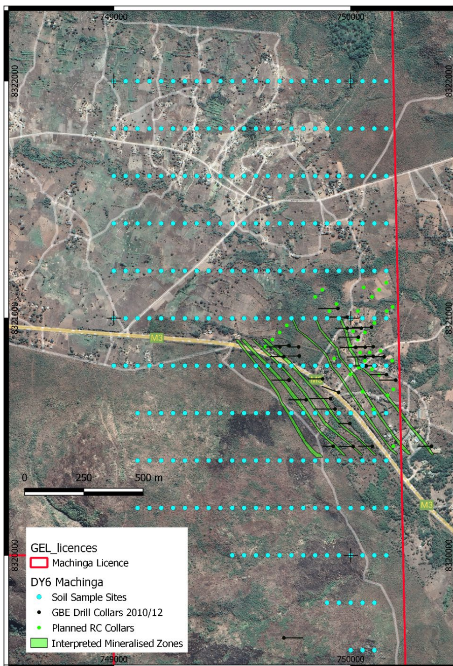
Image 3: Soil Sample locations and Planned Collars for RC Drill Program at Machinga North
