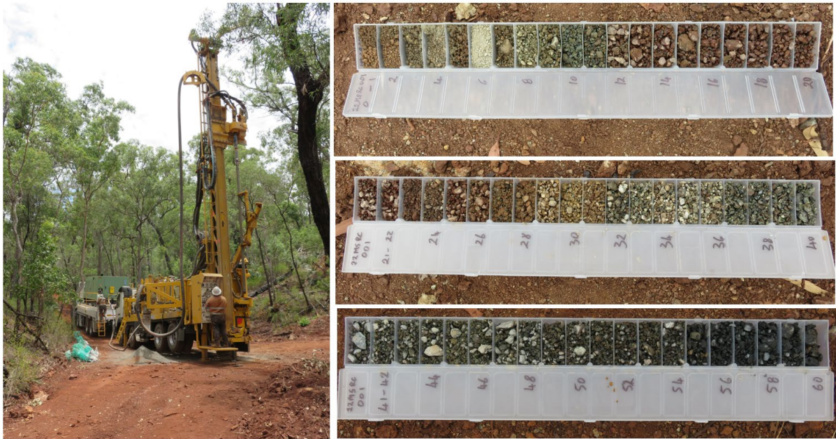
Figure 6: Drill rig operating at Mt Slopeaway in late 2022 (left hand side); representative chip tray samples illustrating lateritic host rock profile in 22msrc001 (right hand side)
