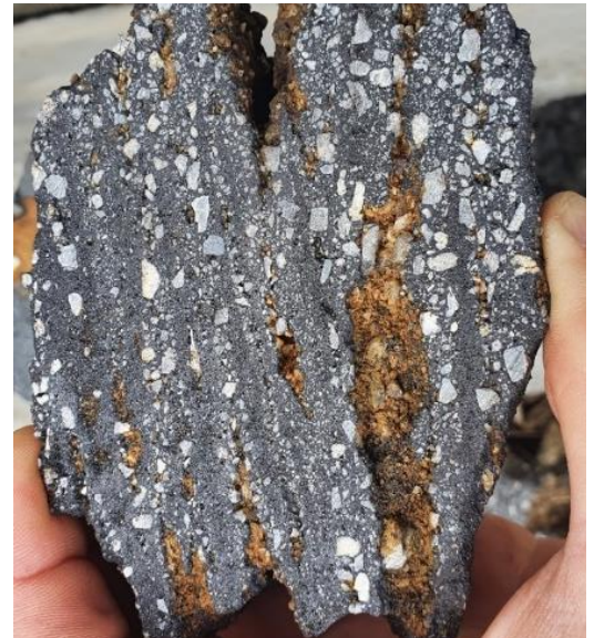
Figure 4: surface sample of cobalt enriched, manganese replacement rock returning 1.19% cobalt, 0.24% nickel and 13.4% manganese
