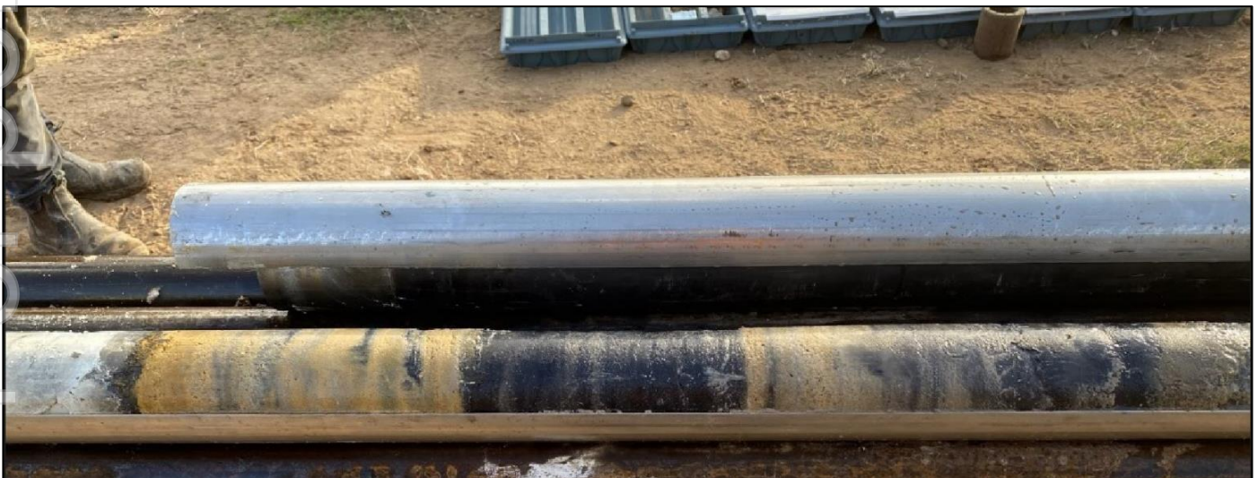
Figure 5: Cobalt in manganese oxide horizon in hole CODD001 returning 1.05m @ 0.252% cobalt at the base of a 12.45m interval of unconsolidated sediments
