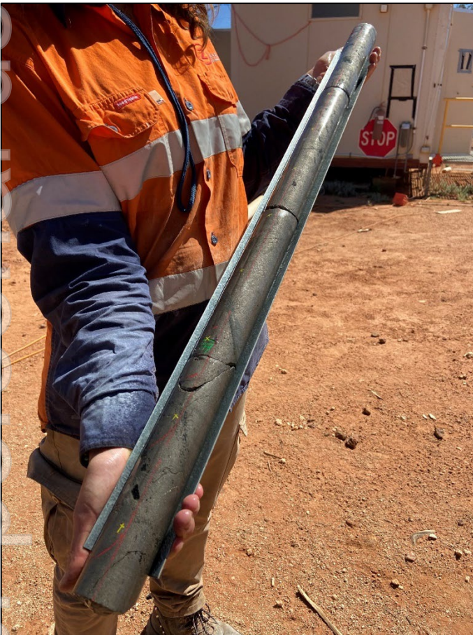
Figure 1: Example of diamond drill core of massive Ni-sulphide intersected in TED54. The section of core in the photograph is approximately 1.0m long and starts from 196.75m downhole. See text for further details.
