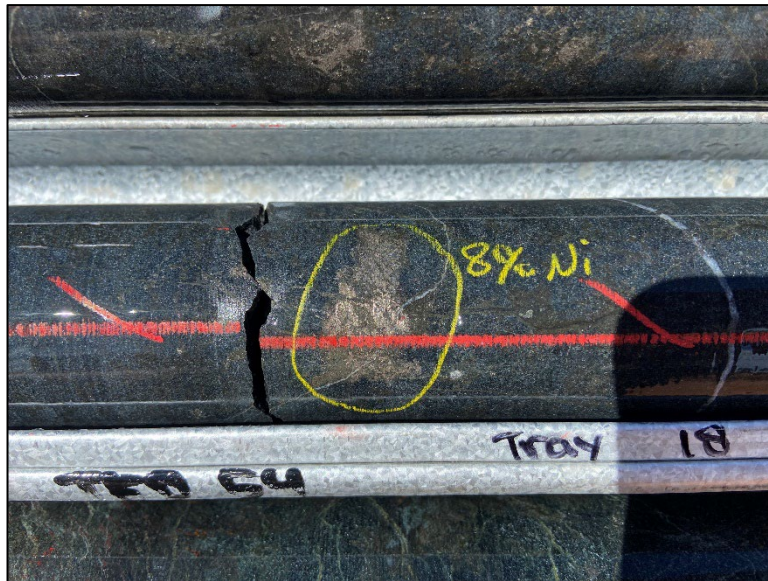
Figure 2: Example of blebby Ni-sulphide in drill core from the 9m blebby Ni-sulphide zone intersected in diamond drill hole TED54 from 162m downhole. The particular focus of the photograph is 167.5m downhole. Note that the Ni-sulphide percentage written on the core is an approximate for the individual bleb only and is from hh-pXRF spot analyses for geologists' use only. This in no way represents the actual average geochemical grade of the rock in the photograph and is an estimation only of the Ni grade of the sulphide minerals inside the yellow circle.
