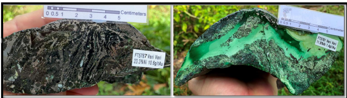
Plate 2: Examples of high grade nickel boudins. Note the curved outer surface, which is typical of boudins formed in shears. The high grade nickel sulphide mineral assemblage is typical of low Fe and low S bearing fluids associated with serpentinisation of ultramafic rocks. Garnierite (vibrant green Ni-Silicate in right photo) is typically found in association with the nickel sulphide and serpentinised shears 3 .
