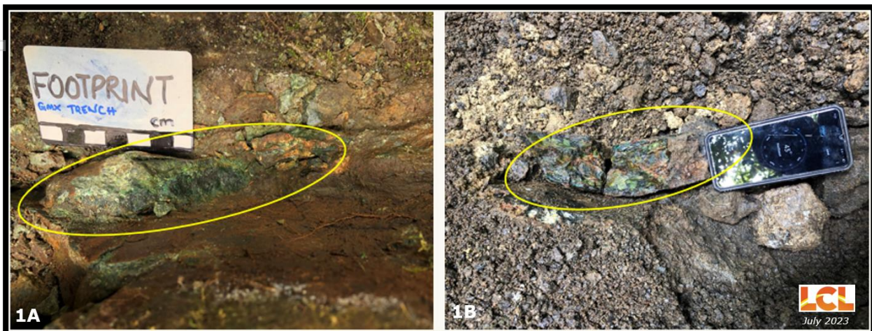
Plate 1: Examples of in-situ boudins of high grade nickel sulphide exposed in pits/trenches. Plate 1B sample 176019: 13.4% Ni, 5.4g/t Au - 10cm x 30cm boudin of NiS, garnierite, magnetite and trace molybdenite hosted in a shear striking 050.
