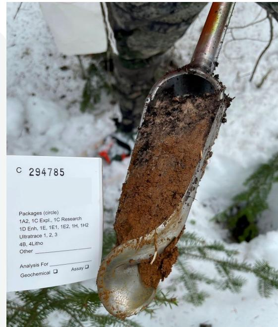
Figure 1 – Hand auger used to collect samples from "B" horizon
