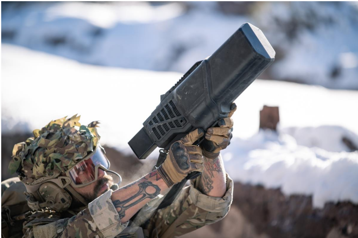
Image: DroneGun Mk4 handheld drone defeat system
