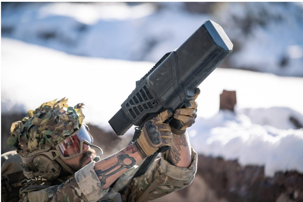
Image: DroneGun Mk4 handheld drone defeat system
