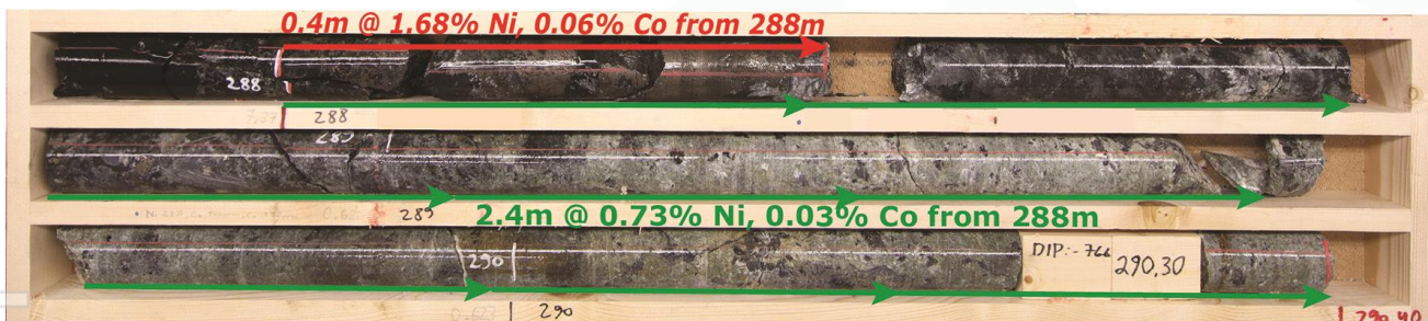
Figure 5. Semi-massive sulphide zone in HOT003, grading 0.4m @ 1.68% Ni, 0.06% Co from 288m, within a broader disseminated sulphide zone grading 20.0m @ 0.26% Ni, 0.01% Co from 284m, including 2.4m @ 0.73% Ni, 0.03% Co from 288m (core size: NQ 32mm diameter).
