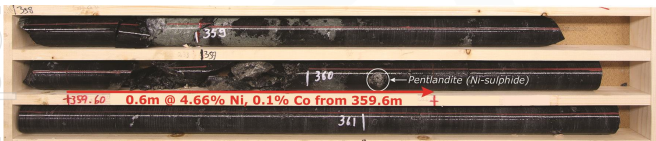
Figure 6. Semi-massive sulphide and blebby Ni-sulphide in HOT006 within broader disseminated sulphide zone grading 25.3m @ 0.29% Ni from 359.6m (core size: NQ 32mm diameter).
