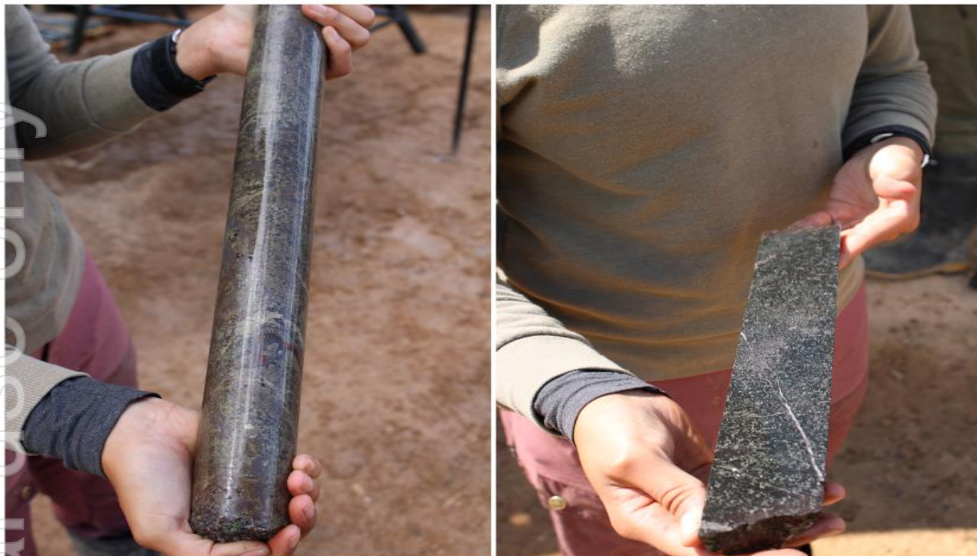
Figure 1: W56 prospect - WL23-367 Massive Sulphides at 227.2m and net texture sulphides at 248.5m.
