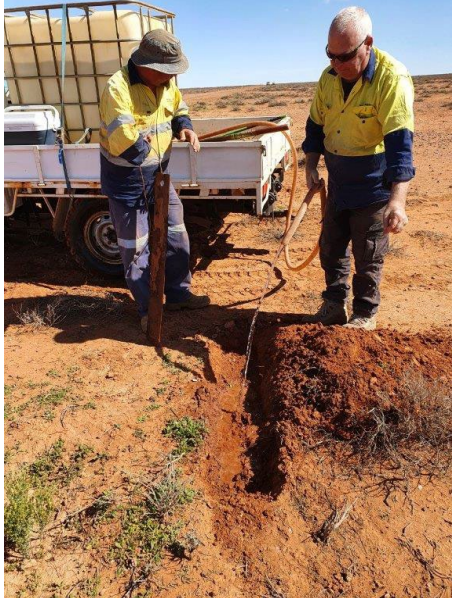
Digging and watering pit for electrode and prepared electrode in the ground
