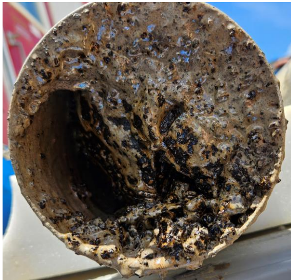
Figure 1 - Core showing the presence of black oil in naturally fractured limestone
