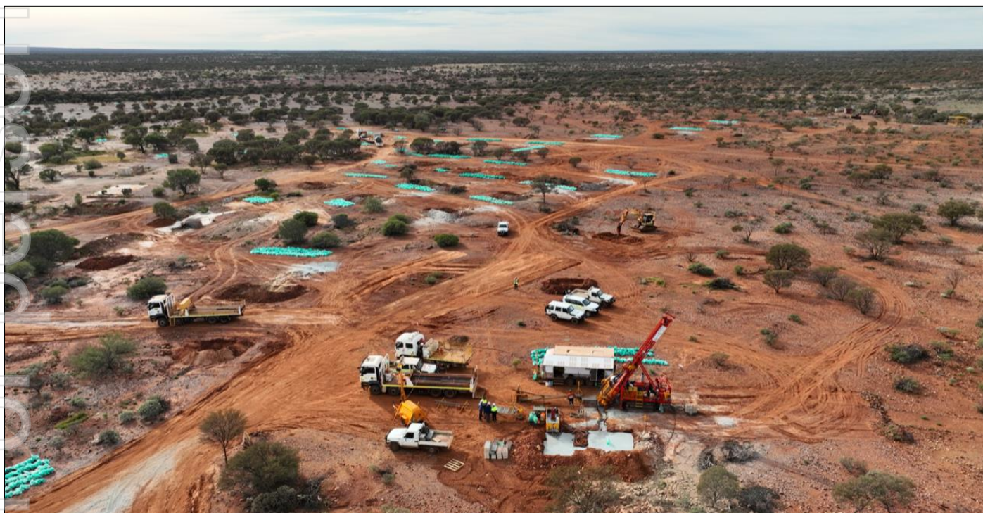
Photo 1 - DDH1 Rig 28 Diamond Drilling at Crown Prince Targeting Depth Extensions to Mineralisation (Recent RC pads can be seen in the background along the line of gold mineralisation)
