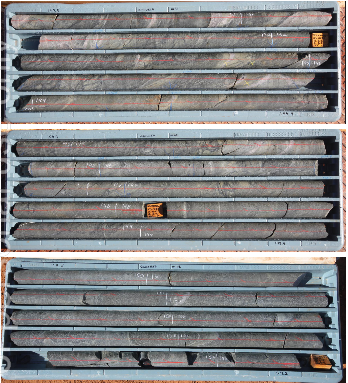
Photo 3 – OGGDD537 Initial core photos showing sheared, quartz-carbonate altered zone (potentially mineralised) from 140.3m to 148m. This interval is down dip of the high-grade shallow RC intercepts discussed in this release. Assays pending. Interval from 150m onwards less altered and unlikely mineralised. Assays pending.
