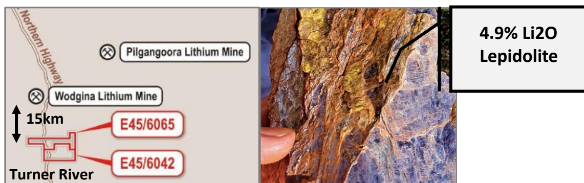
Figure 1: Location map of QXR’s Turner River project licences relative to large Pilbara lithium mines, and photo of weathered lepidolite in rock samples from the drilling area shown in Figure 2,3.
