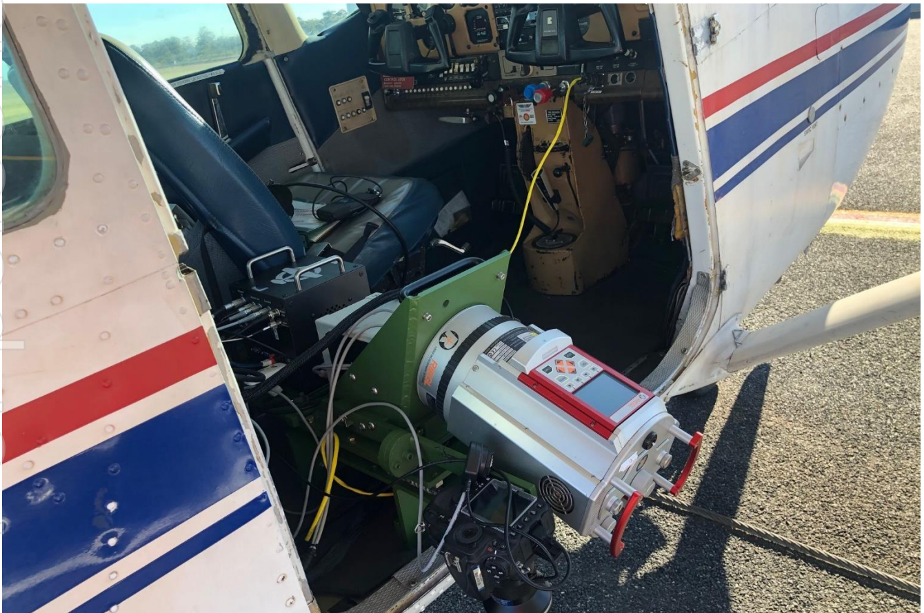
Figure 1: Airborne LiDAR system used for the survey.
