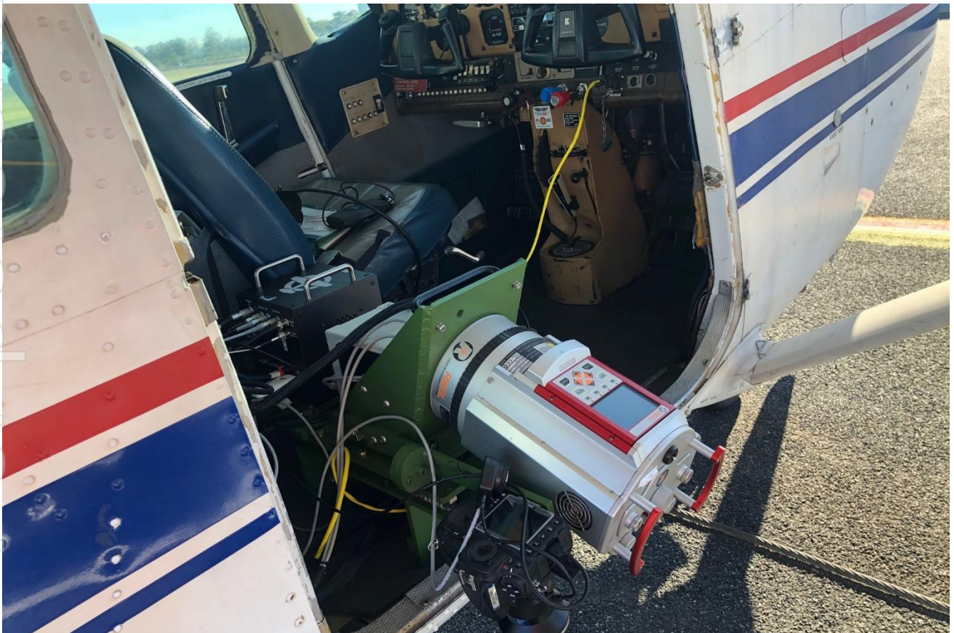
Figure 1: Airborne LiDAR system used for the survey.
